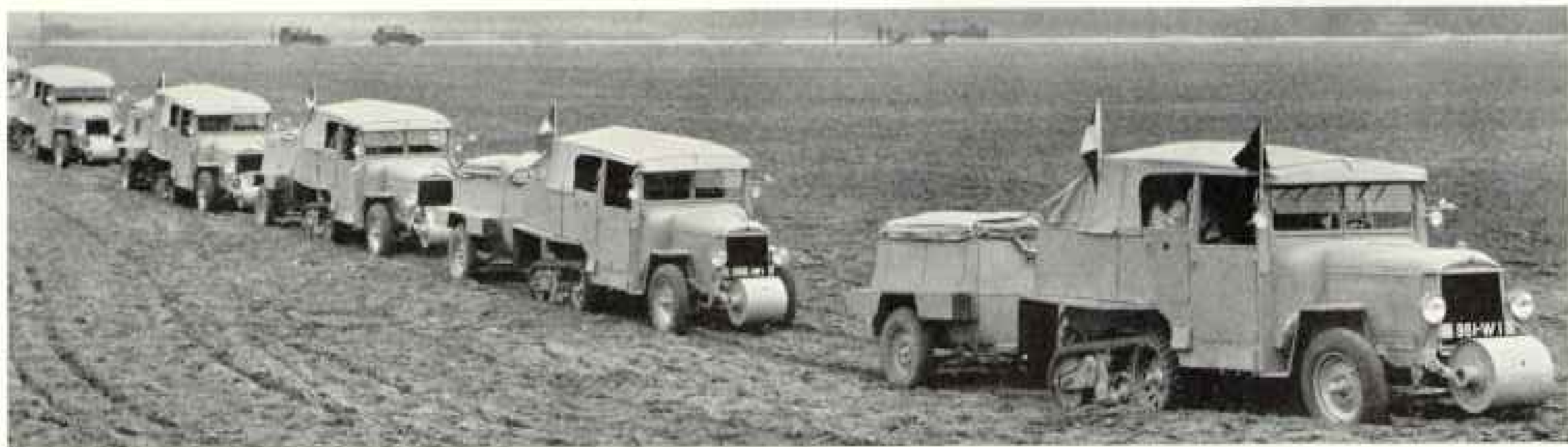
A BIT OF HEAVY GOING NEAR FONTAINEBLEAU SERVES TO PROVE THE EFFICIENCY OF THE TRACK-TYPE CARS
