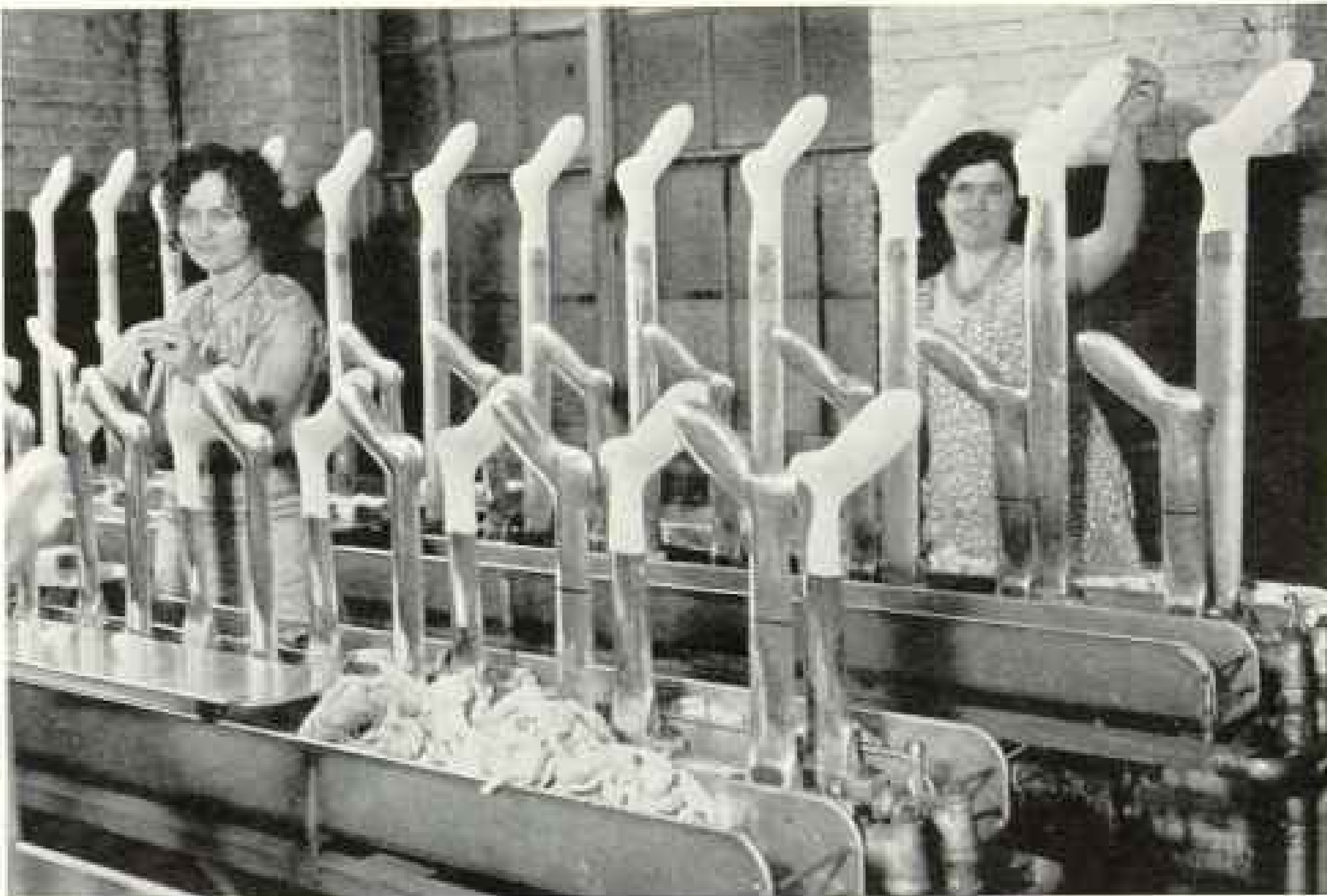
HOLLOW, STEAM-HEATED, ALUMINUM FEET, USED FOR IRONING AND DRYING SOCKS. The newly knitted socks and anklets are washed and then stretched over these models. A hosiery mill in Anniston (see, also, Color Plate X).
