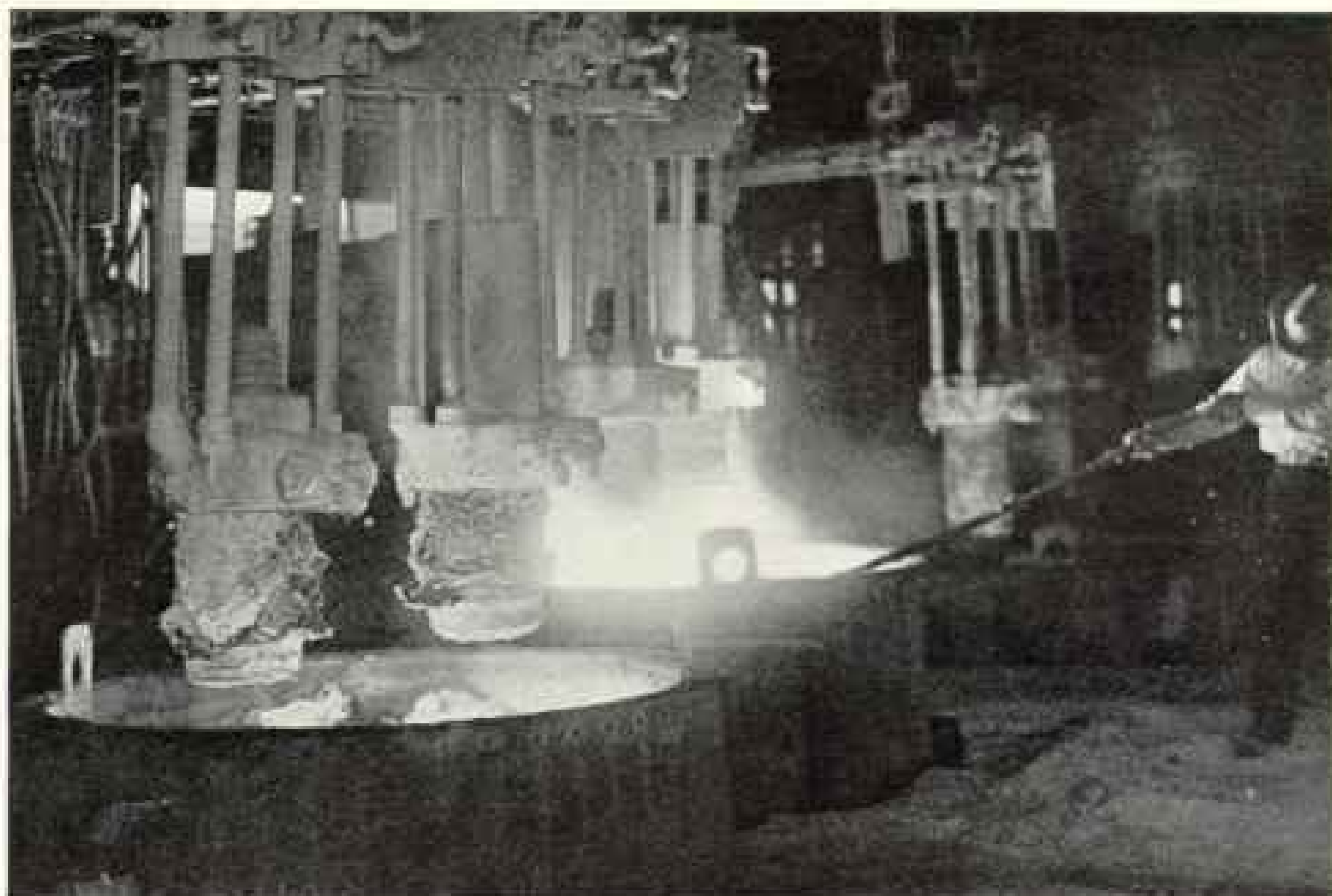
FURNACES AT ANNISTON FOR SMELTING BAUXITE AND MAKING ALUMINOUS ABRASIVE MATERIAL.
