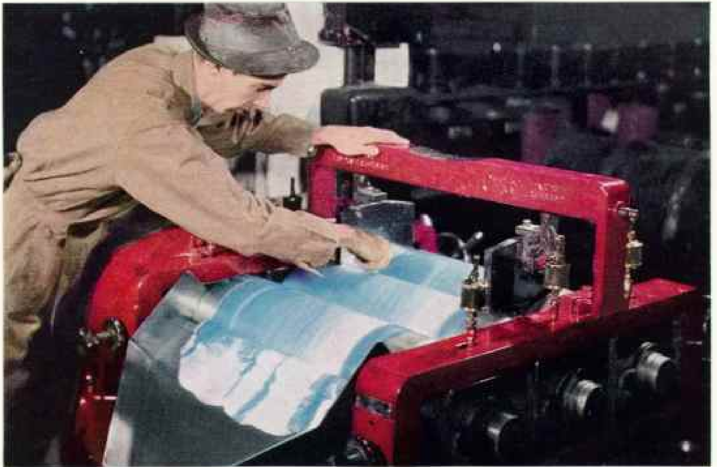
Ink for Paper Cartons Flows from a Three-roller Mill in Washington, D. C. With a spatula, the mill hand keeps this mineral oil and rosin varnish ink flowing smoothly.
