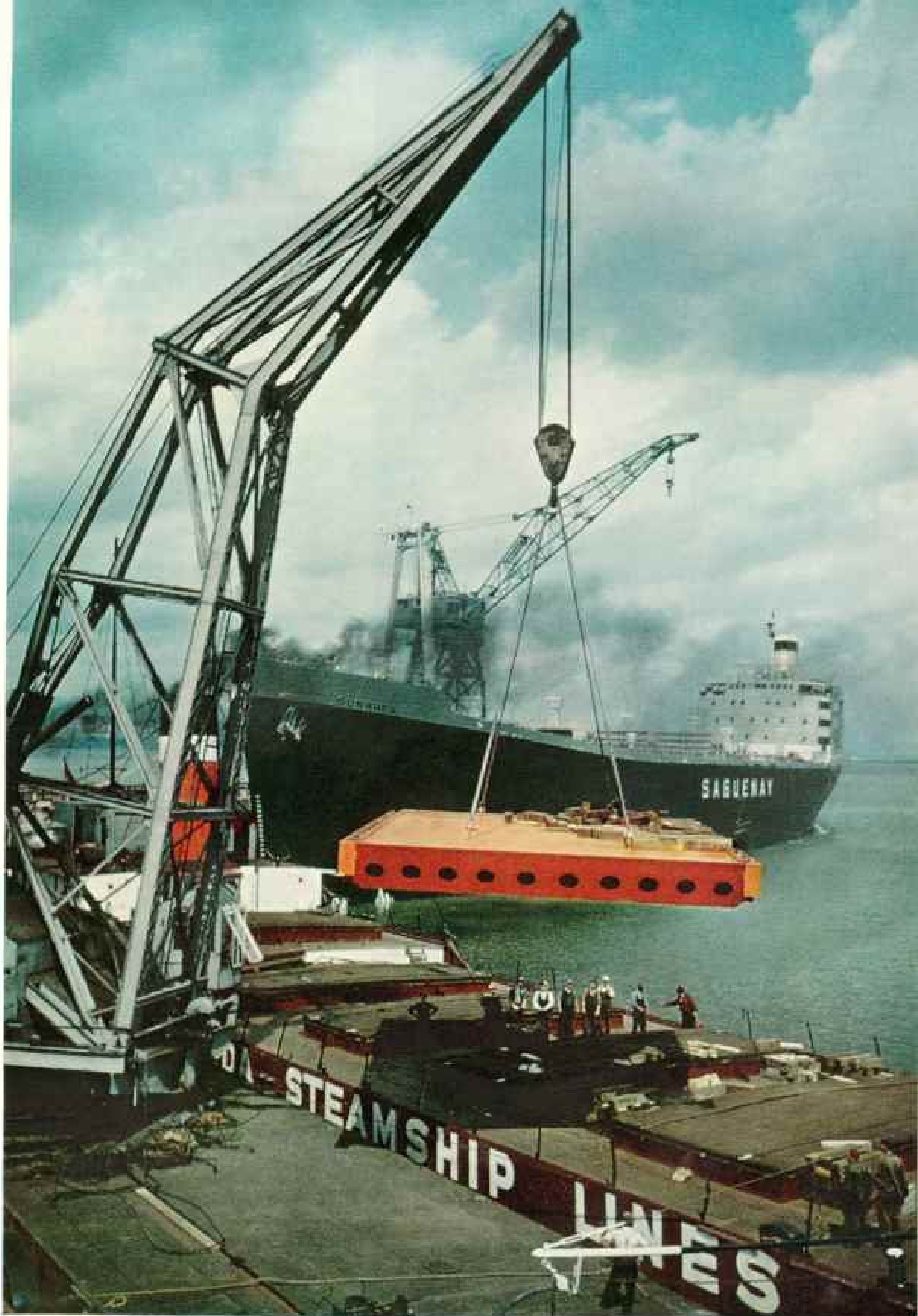
Gantry crane at Lauzon, Quebec, loads a 45-ton gate for the powerdam at Beauharnois. Newly launched, the Saguenay line's freighter Sarthea carries an all-aluminum superstructure.
