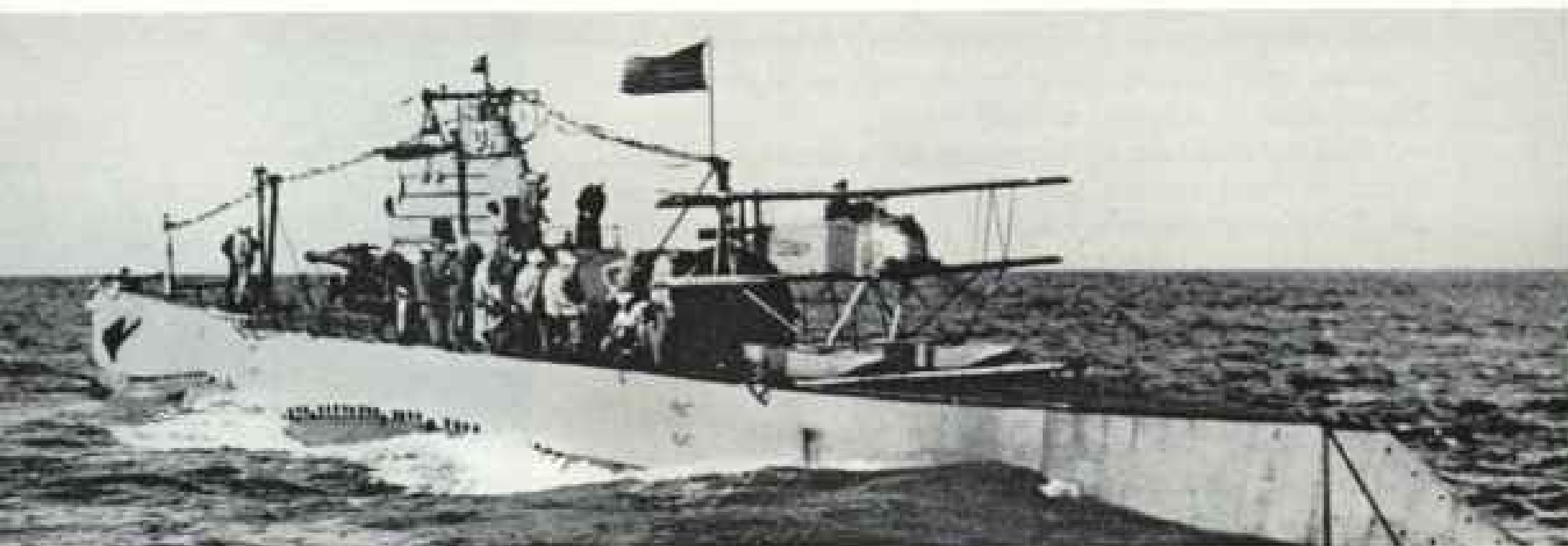
Novel experiment in 1926 saw the submarine S-1 launch a Cox-Klemin XS-2 seaplane off New London, Connecticut. Disassembled, the plane rode in a waterproof tank amidships. Within 12 minutes after the sub surfaced, crewmen could assemble the plane, put it in the water, and watch it take off. To retrieve the plane and submerge again required but 13 minutes.
