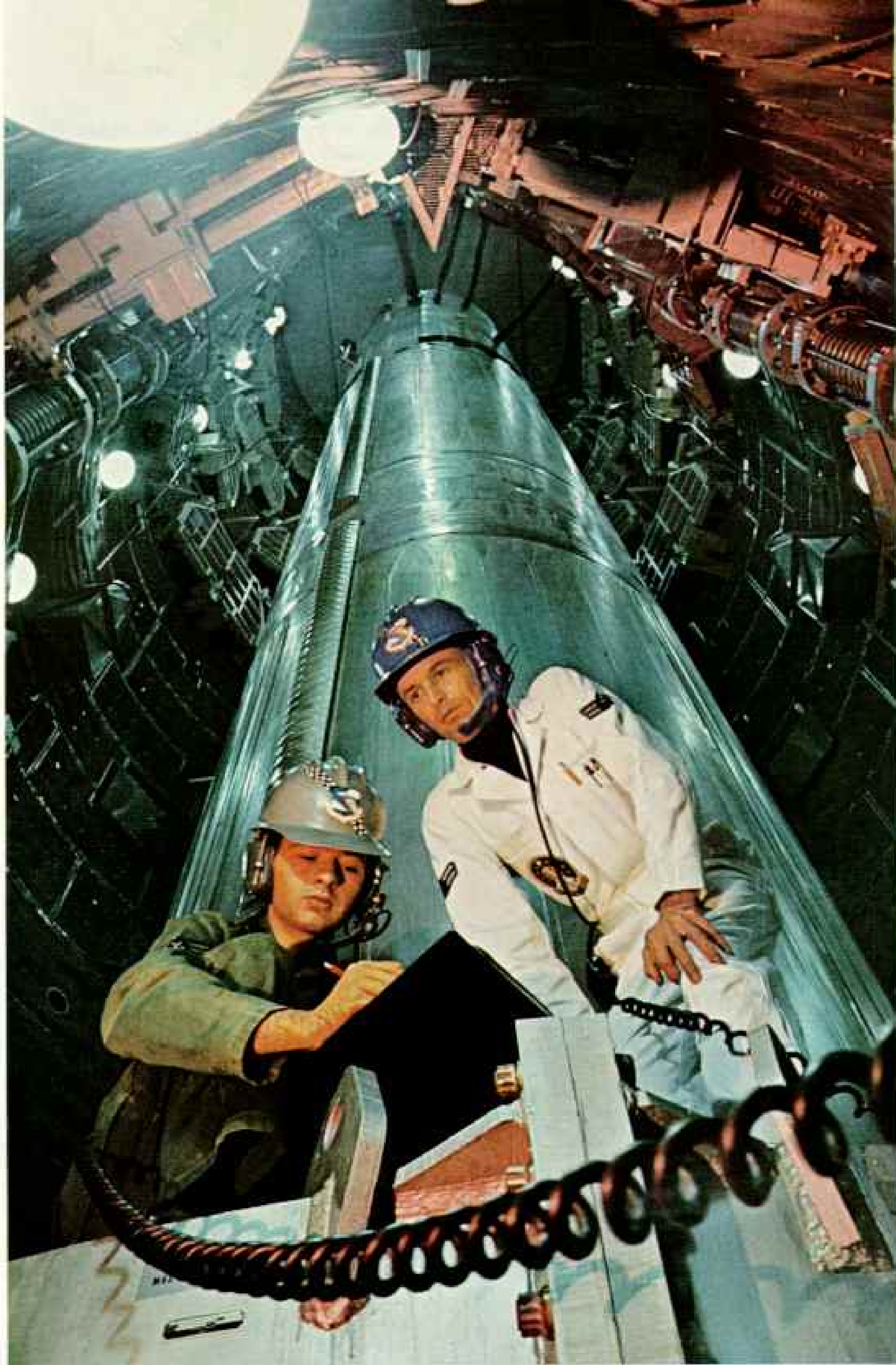
Mightiest U. S. military missile, Titan II stands ready for instant action at Little Rock Air Force Base, Arkansas. With propellants that ignite on contact, the missile can fire within seconds after its silo cover opens. Titan II puts Gemini into orbit; a Titan III may propel MOL into space.
