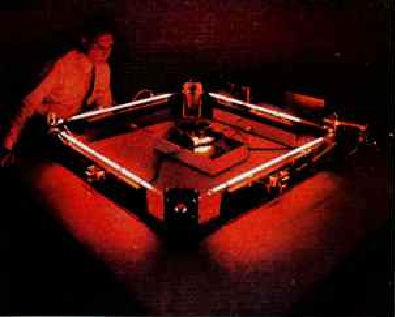
Ring laser, two beams traveling in opposite directions around a closed path, acts like a gyroscope, sensing changes in direction.
