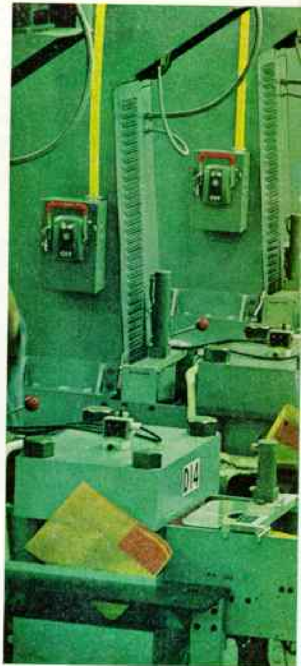
Music maid at the Capitol Records plant in Winchester oversees a battery of automatic stamping machines; each presses 100 discs an hour, here the
