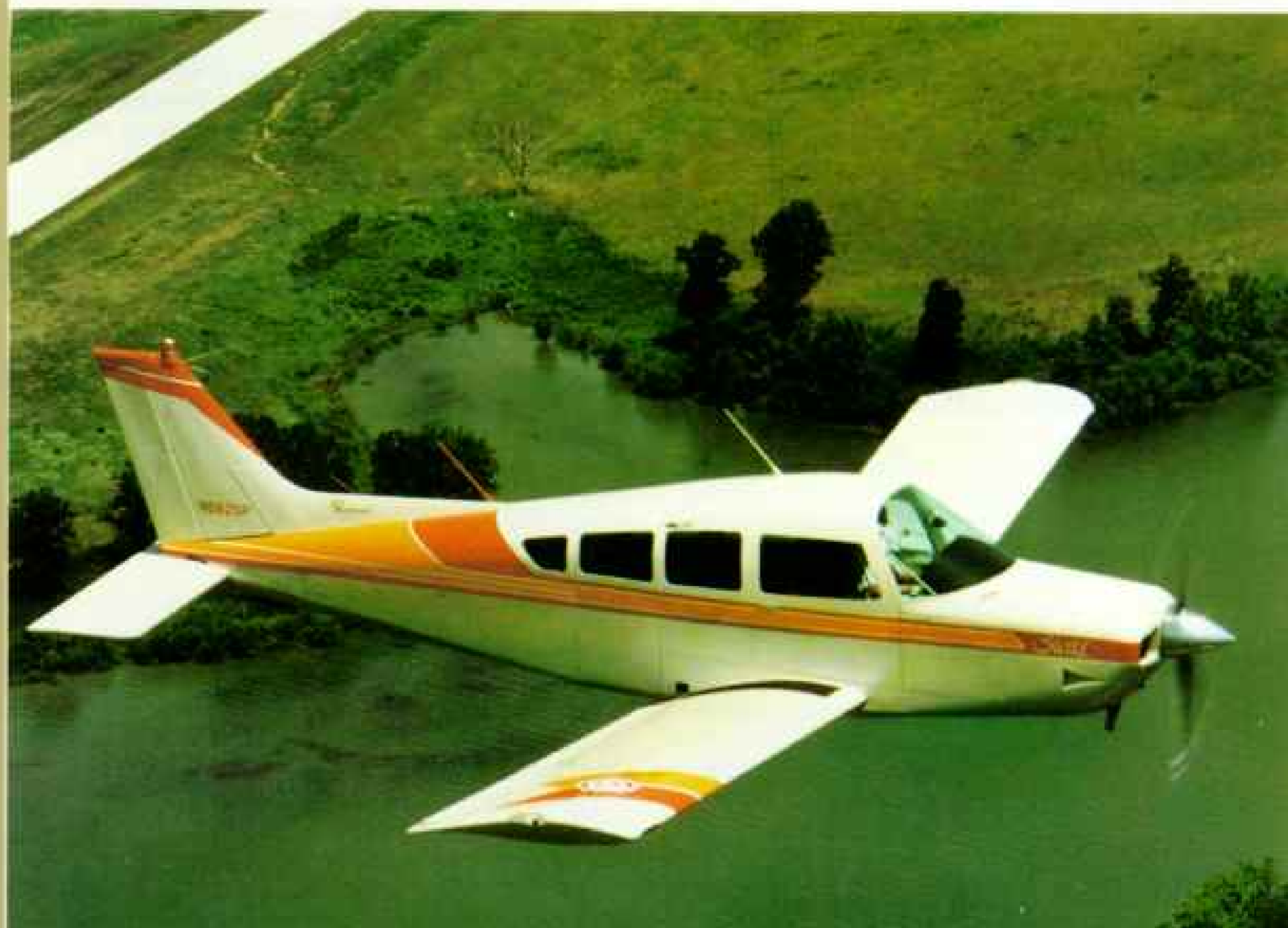
The Beechcraft Sierra. A fuel efficient single engine aircraft that can carry 4 people nearly 800 miles nonstop at over 160 mph.
