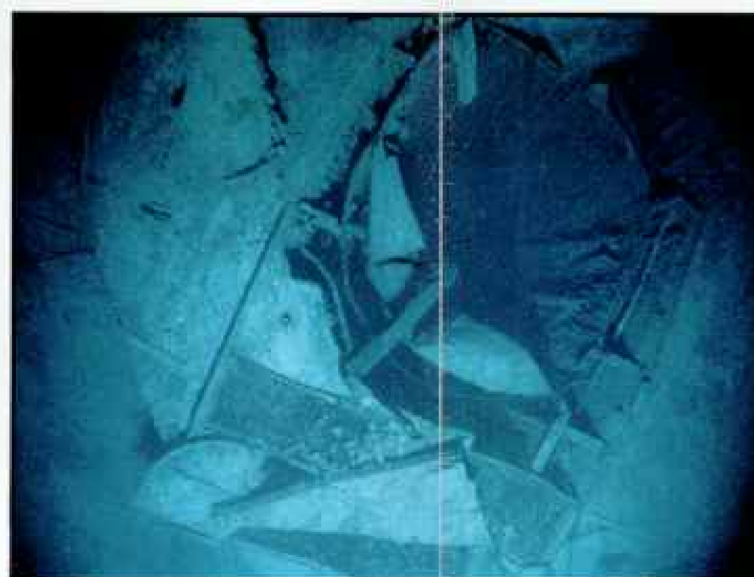
8 Jagged metal surrounds the hole left where the number one funnel tore loose.
