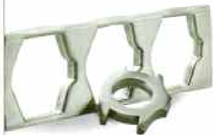
Every Oyster case is hewn from a solid ingot of stainless steel, 18kt gold or platinum.
