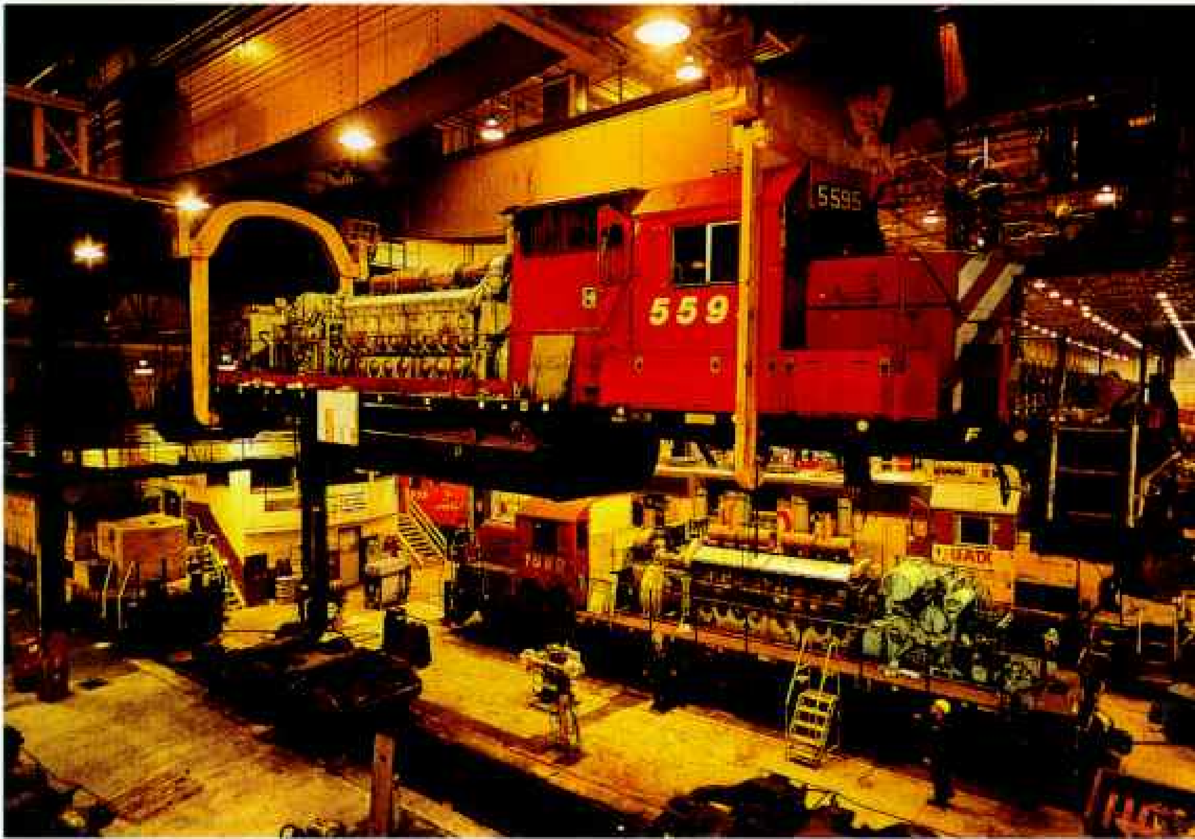
Up but nowhere near running, a 200-ton locomotive receives an overhaul at the Ogden Diesel Shop in Calgary. Every five years or one million miles it gets the same treatment, which can keep it rolling for 20 years or more.
