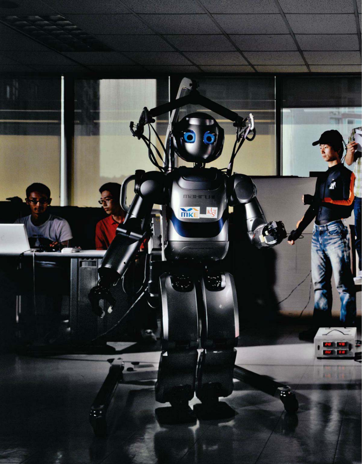
Domestic robots keep busy at the Korea Institute of Science and Technology. One makes toast, while the appropriately attired bot at right waits to deliver the toast to a human. At left, a third robot tests technology for navigating through a house, controlled by the movements of the researcher in the baseball cap.
