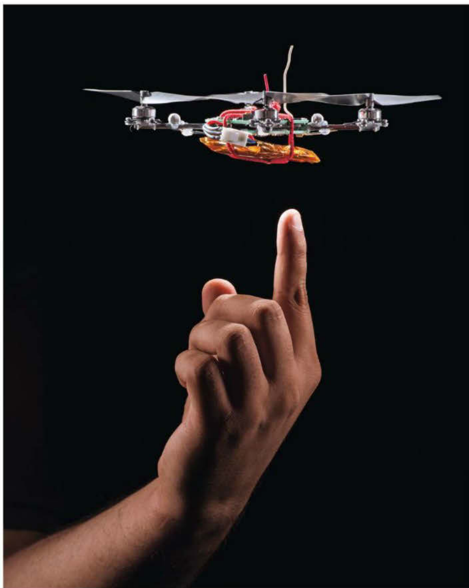
This “micro air vehicle” with four rotors, made by KMeI Robotics in Pennsylvania, can fly in swarms with its mates. The drones navigate autonomously, without a pilot.
