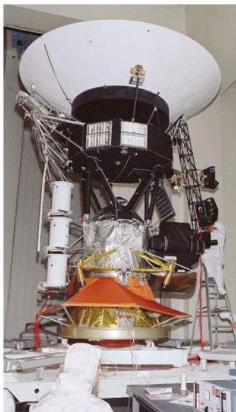
A Voyager spacecraft undergoes testing at JPL in November 1976, nine months before its launch. Originally built to last five years and explore Jupiter, Saturn, and their moons, the Voyagers are now far beyond Pluto and still sending scientific information back to Earth.
