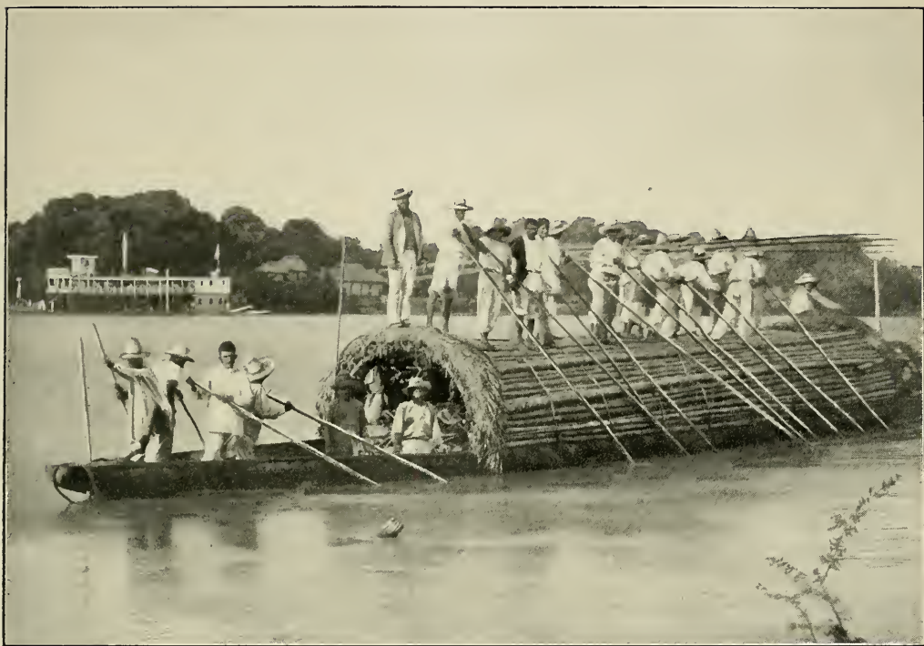
Hand Propelled Freight Boat for Shallow Tributaries of Magdalena—Large river steamer in background
