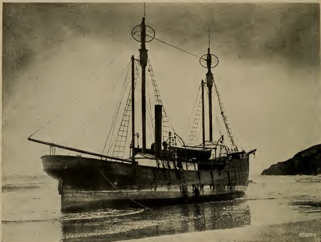
THE COLUMBIA RIVER LIGHT VESSEL, AFTER BEING STRANDED ON CAPE DISAPPOINTMENT IN 1899, WAS HAULED THROUGH THE WOODS 700 YARDS AND LAUNCHED INTO THE RIVER (SEE PAGE 43)
