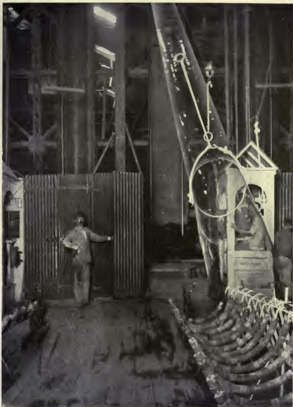
A MACHINE-BLOWN CYLINDER OF WINDOW GLASS BEING LOWERED INTO ITS CRADLE
