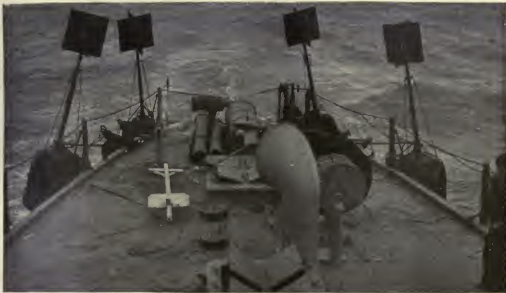
A VIEW OF THE STERN OF THE U. S. S. "BALTIMORE," SHOWING MUCH OF THE PARAPHERNALIA WITH WHICH A MINE-LAYER IS EQUIPPED
