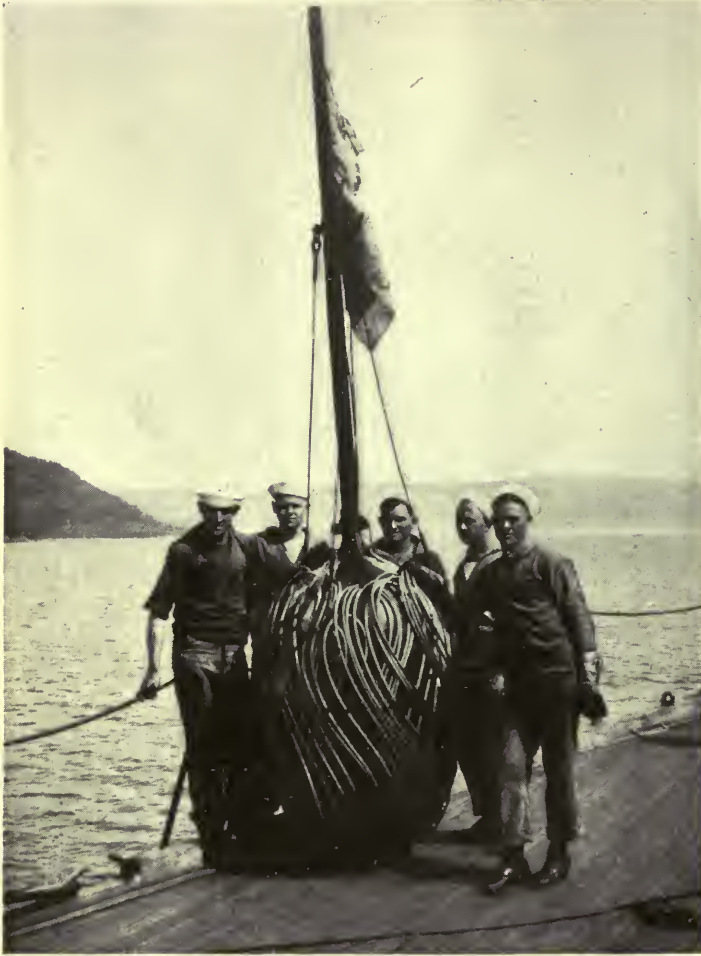
A BUOY READY TO BE LOWERED INTO THE SEA TO MARK THE LIMIT OF A MINE FIELD
