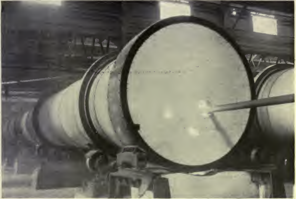
A ROTARY CEMENT KILN
