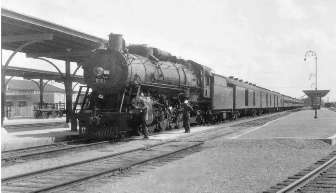
The Meteor was another member of the Frisco's premium fleet of trains. It ran between St. Louis, Tulsa, and Oklahoma City on an overnight schedule. Here, Frisco's No. 1518, a Mountain type, prepares to depart Oklahoma City Union Station with the Meteor in the 1940s. Frisco photo, author collection
