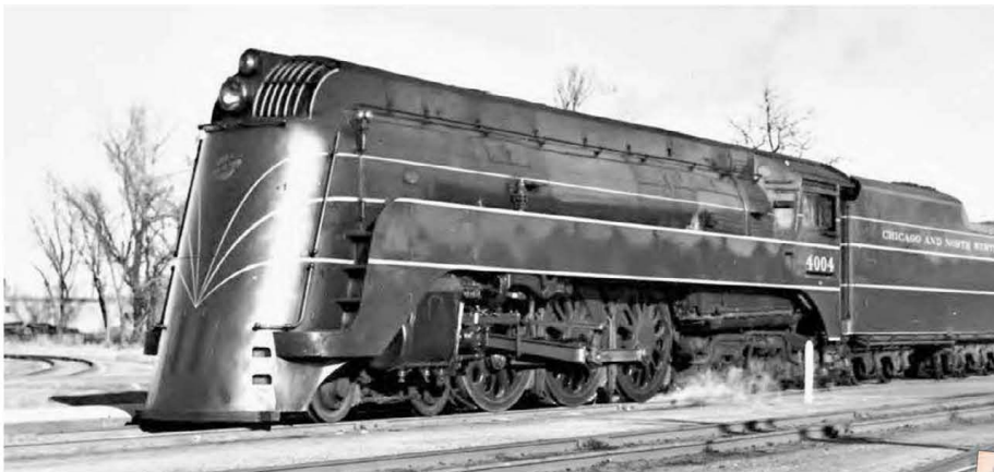
No. 4004 was one of nine green and gold streamlined 4-6-4 Hudson-type locomotives built by Alco for the Chicago & North Western in 1938. Designated Class E-4, the locomotives were considered for the line's elite 400 but instead were utilized on the Chicago-Omaha Overland Route trains. Author collection
