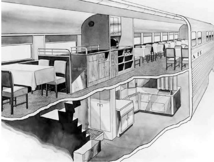
A builder's cutaway illustrates the two levels of the Hi-Level dining cars built for El Capitan . Santa Fe drawing, author collection
