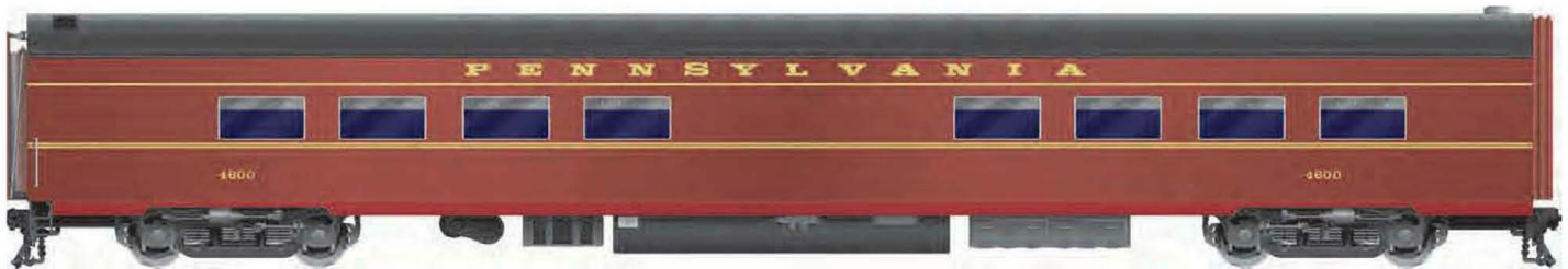
Pennsylvania's Broadway Limited featured five 68-seat dining cars (Nos. 4600, 4602, 4604, 4606, and 4608), each with a four-seat waiting lounge. They were built by American Car & Foundry and delivered in 1949.
