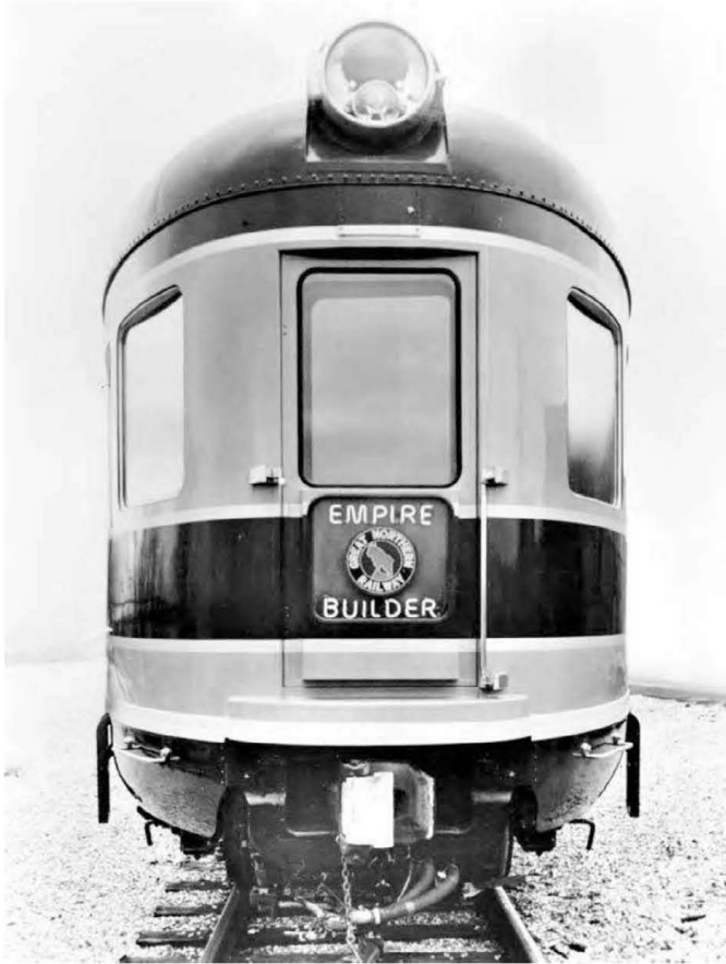
An Empire Builder tail sign adorns the rear of one of the Great Northern's sleeper-observation-lounge cars built by American Car & Foundry in 1951. The cars had extended-height windows in the observation-lounge end. Great Northern photo, author collection
