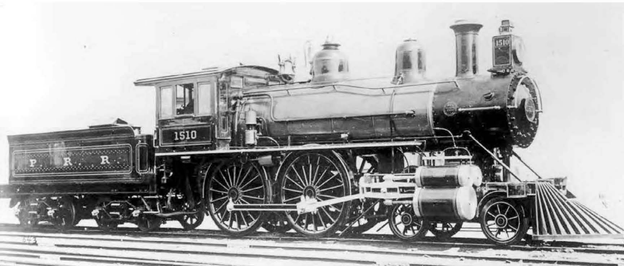
Pennsylvania 4-4-0 American-type locomotive No. 1510, Class D61, was an experimental unit built by Baldwin in 1892. No. 1510 was a good example of the Pennsylvania Railroad's efforts in the development of locomotive technology. The engine had experimental Vaucain compound cylinders and 68-inch driving wheels. It was retired in 1911.
