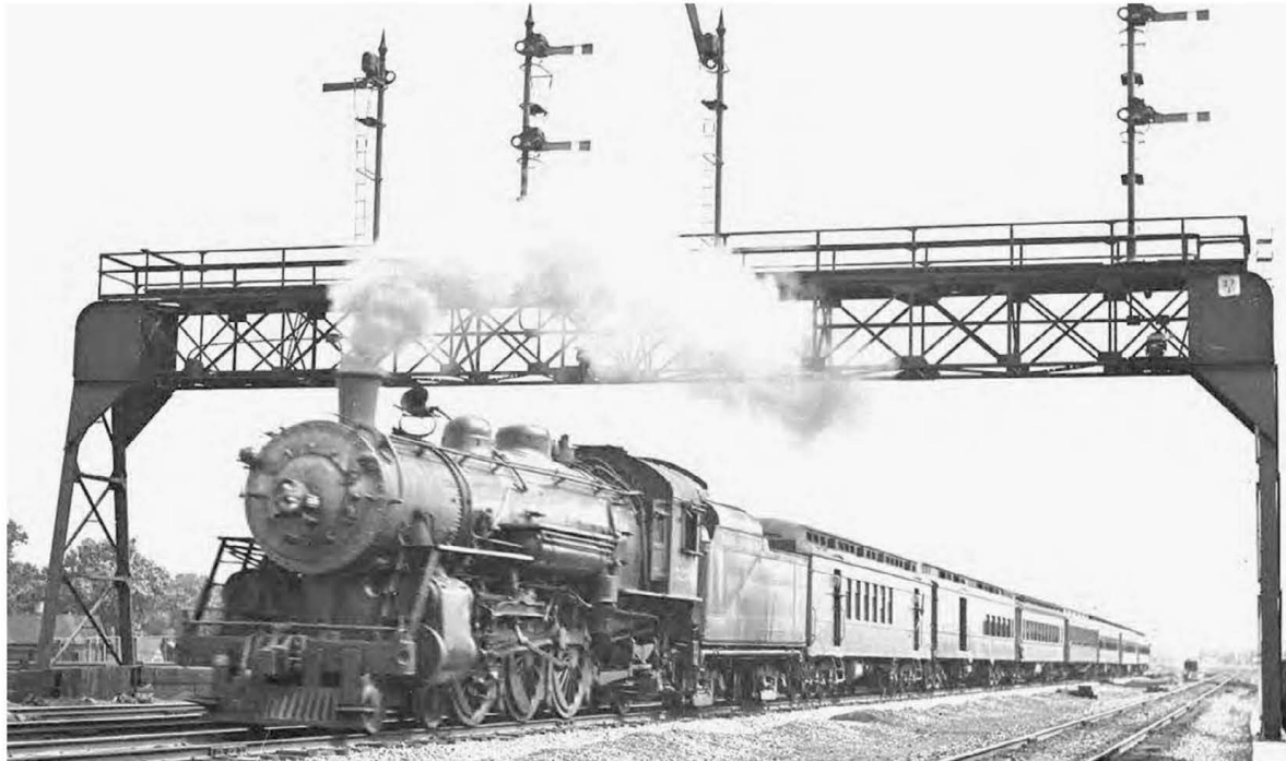
Led by a heavy Pacific, the Alton Limited approaches Joliet, Illinois, in June 1932. Between 1935 and 1938, six of these locomotives were modernized and designated Class P-16. These were the heaviest Pacifics on the Alton. In their prime the boilers, cylinder jackets, and tenders were painted maroon with gold striping. DeGoyler Library, Southern Methodist University, Dallas, Texas, Ag1982.0231
