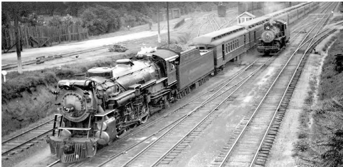
Southern Railway 4-6-2 Pacific No. 1394 heads the nine cars of the Crescent Limited at Spartanburg, South Carolina, on August 5, 1932. Otto Perry, Denver Public Library, Western History Collection, Neg. OP-15261
