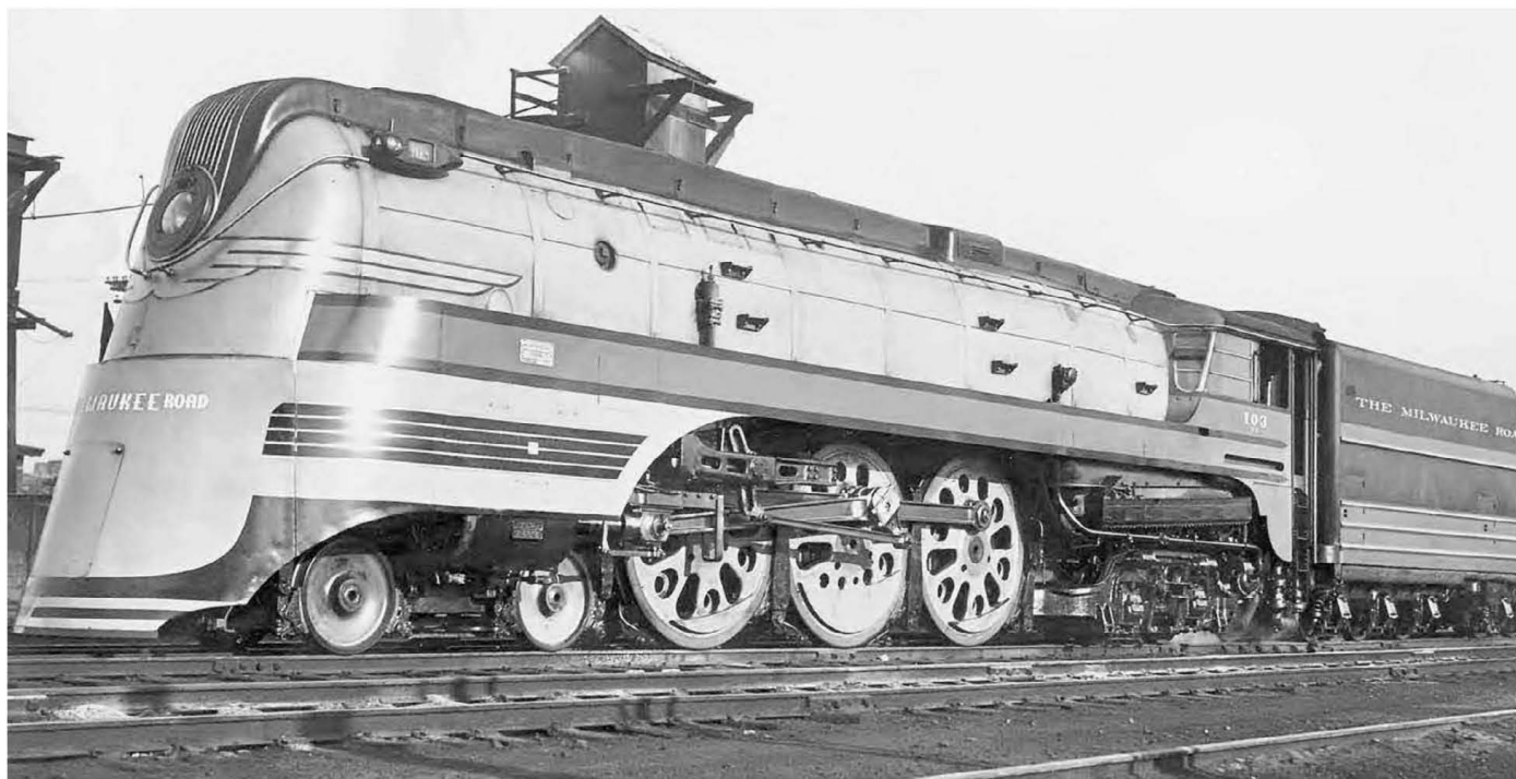
Milwaukee Road F-7 Class 4-6-4 locomotive No. 103 at Chicago, Illinois, on November 25, 1938. Jay Williams collection
