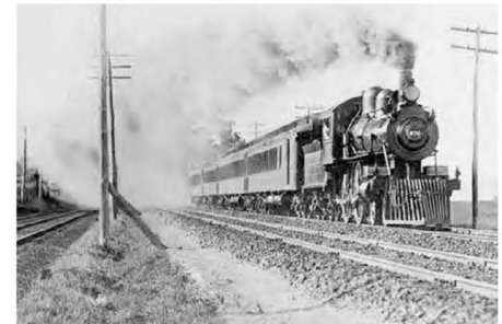
Locomotive No. 870 charges down the line at the head of a four-car Empire State Express in the mid-1890s. The locomotive was a 4-4-0 type and had been in charge of the inaugural Empire State Express on October 21, 1891. That train made a record-setting run between New York City and Albany, New York, when it traveled 143 miles in 183 minutes. Locomotives such as Nos. 999 and 870 helped establish the Empire State Express , at the time one of the world's fastest scheduled passenger trains. Andrew Merriees, Library and Archives Canada, Neg. No. PA-181397
