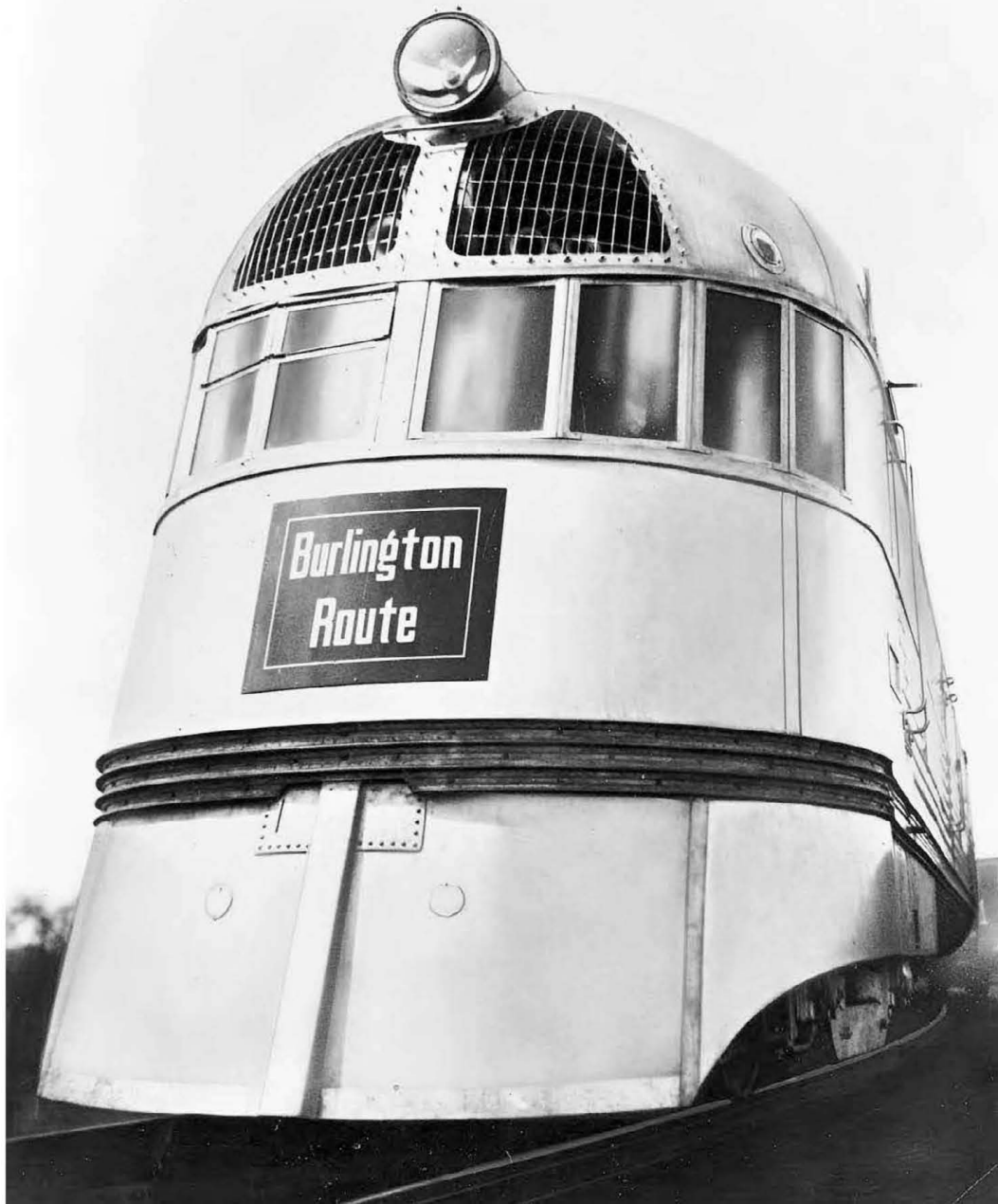
The Pioneer Zephyr was America's first diesel-powered, stainless-steel streamliner. CB&Q photo, author collection
