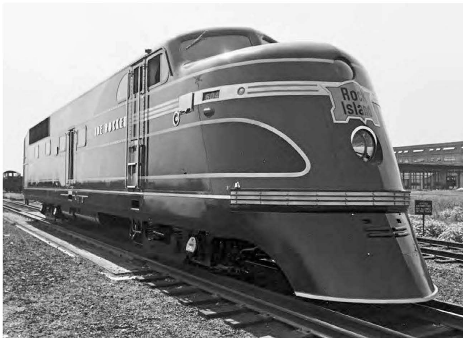
The six TA-class locomotives built by EMC in 1937 to power the Rock Island's Rocket trains incorporated the cab above a rounded nose-carbody truss construction introduced that year on Electro-Motive's E units. EMC photo, author collection
