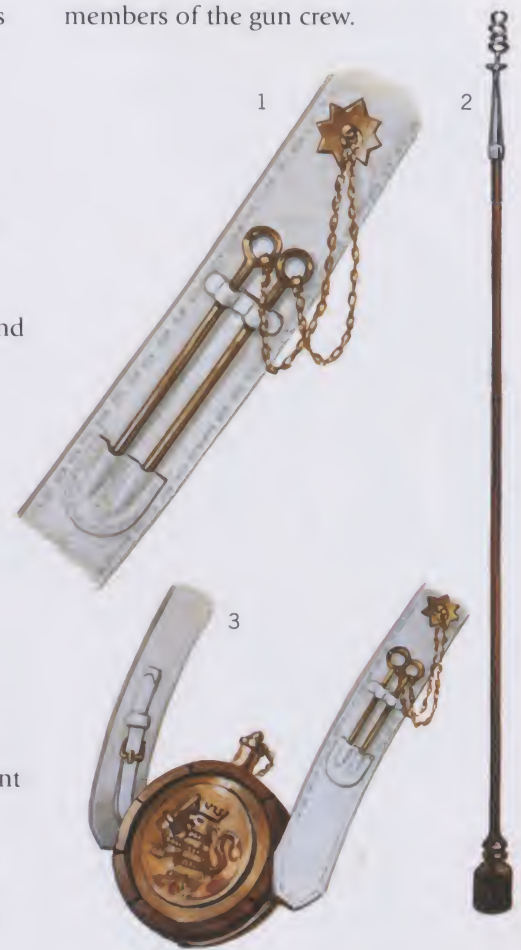
▲ GUNNER KIT 1 Detail of gunner's picker, for clearing the touch-hole and piercing the bagged charge or the cartridges. 2 The combined rammer/extraction tool. This could be used to load the gun and to extract any ball or cartridge if it was decided not to fire the piece after it had been loaded. 3 Detail of a Hessian gunner's powder flask, embossed with the rampant Hessian lion.
