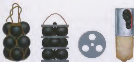
▲ Artillery anti-personnel ammunition, grapeshot on the left, canister on the right.
