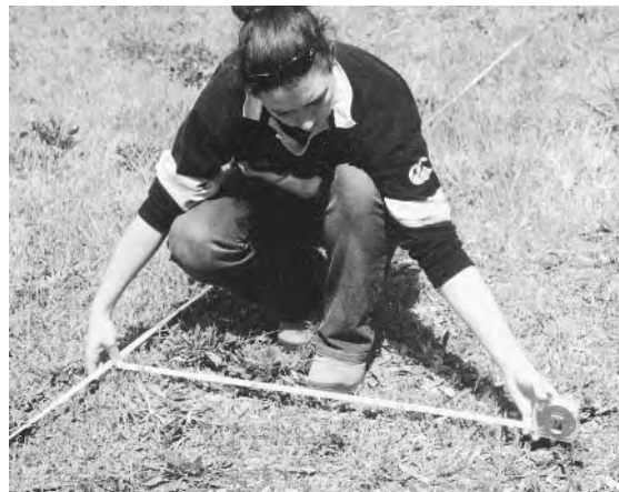
FIGURE 4.5: Over a short distance (less than 3 metres), you can estimate a right angle for an offset reasonably accurately by eye, but only from the position of the baseline
