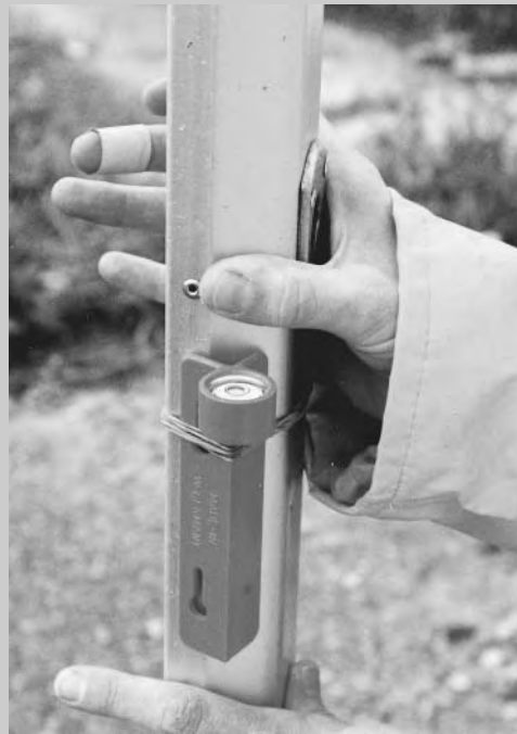
FIGURE 4.16: Using a spirit level to check whether the stadia rod (levelling staff) is vertical
