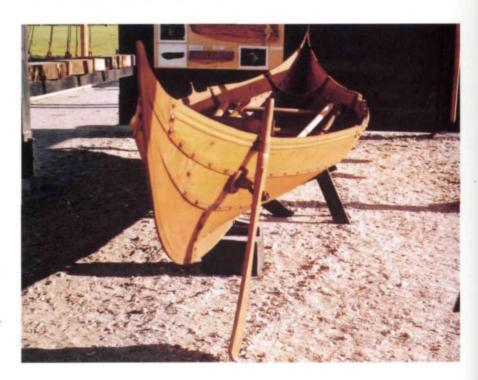
This small boat, built in the Museum shipyard at Roskilde, is a replica of one of the three boats interred with the Gokstad ship. Lightly constructed, it shares the same gracious lines as the parent ship. In parts of Scandinavia, similar vessels are in use to this day. (Keith Durham)
