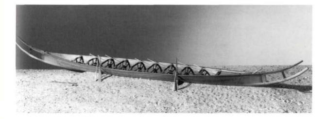
overall structure of the vessel, would continue well into the 10th century. Spanning these ribs are thwarts for the crew, which are angled in such a way as to maximize the power of a downward paddle thrust. The double row of props supporting them further strengthens the thinly planked hull.
