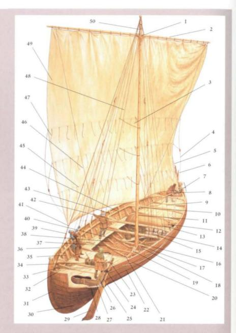
An IIth-century knarr as she would have appeared en route to Iceland. Note the exposed conditions that had to be endured on these long voyages by crew and passengers alike. A crew member deploys the beiti-ass. Note the ship's boat lashed across the cargo hold. In addition to cargo, Norse vessels would invariably carry some form of ballast. In order to show the interior of the ship clearly, this has been omitted from the illustration. (Steve Noon © Osprey Publishing Ltd)
