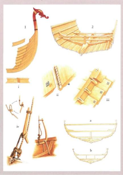
Left to right: (i) scarf joint, (ii) rove, rivet and tarred rope, (iii) rib, clinker-built strakes and trenails. (iv) shows two kinds of shroud-pin or vantnäle and the manner in which they are used to secure the shrouds to the hull.
