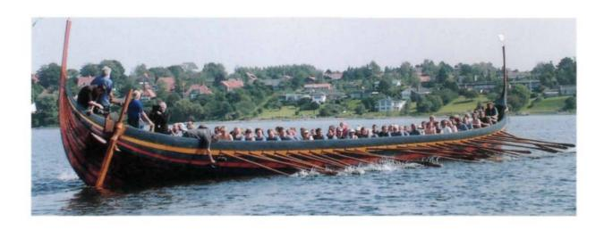
of iron, which was used to manufacture the ship's 7,000 nails. Linden bast, horsehair and hemp were used in the manufacture of the ship's 2,000 metres (6,562 feet) of cordage and the II8-square-metre (I270-square-feet) sail was manufactured from flax.
