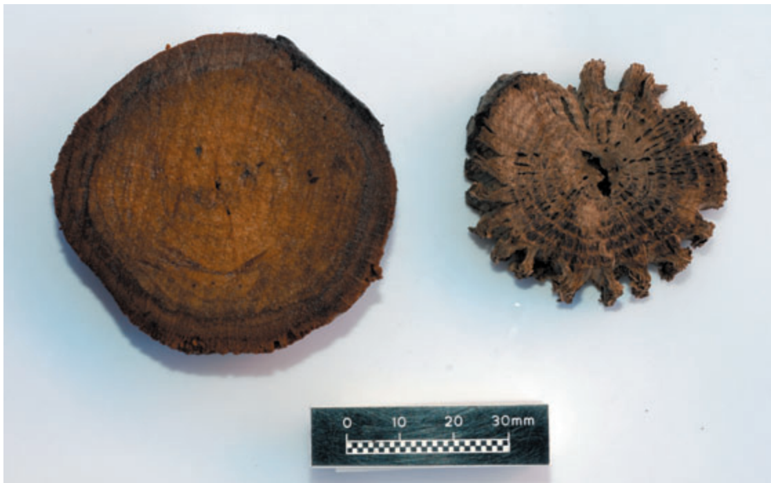
Plate 16.1 Samples of oak from the Mary Rose . The one on the left is untreated and wet. Following drying, the sample on the right has suffered large volumetric shrinkage, indicating the need to stabilize with polyethylene glycol prior to drying. (Photo: Mary Rose Trust)
