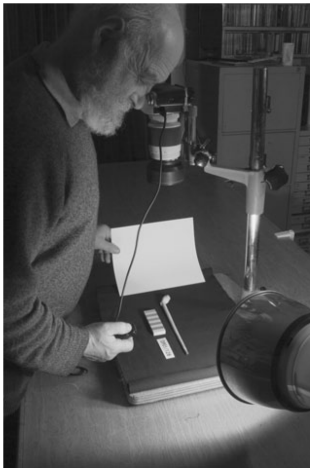
Figure 10.2 A simple set-up for photographing finds using a vertical stand. The white clay pipe has been set on a matt black background, with a scale and reference number appropriately placed. A single light source has been augmented by a white card reflector to 'kick' light back into the shadow side so as not to obscure the edge of the object. A remote release is being used to avoid camera shake. (Photo: Edward Martin)
