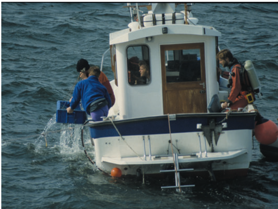
Plate 6.2 A commercial archaeological diving unit working to UK Health and Safety Executive protocols for surface-supplied diving. The supervisor is in the cabin, where he is in voice communication with the diver, whose progress he monitors via a helmet-mounted video link. A tender monitors the diver's umbilical, while behind is the standby diver, fully kitted-up except for his mask. (Photo: Colin Martin)
