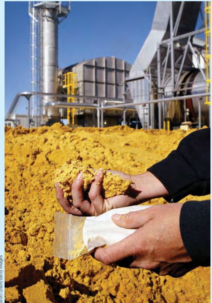
● Figure 11.B Pictured here is a byproduct of corn ethanol production, which can be combined with other ingredients to make high protein livestock feed.
