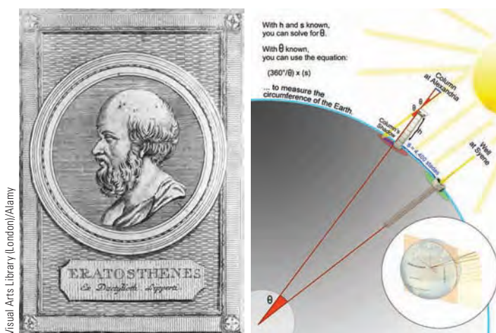
• Figure 1.1 By measuring the lengths of shadows in the Egyptian cities of Alexandria and Aswan (Syene) and applying a simple mathematical formula, the Greek geographer Eratosthenes—the first person known to use the term geography —was able in the 3rd century B.C.E. to determine the circumference of the earth as 252,000 stadia—between 24,660 and 28,965 miles (39,690 and 46,620 km; we are not certain of the length of his stadion). The circumference of the earth, measured around the poles, is recognized today as 24,901 miles (40,075 km); Eratosthenes was right “in the ballpark”—not bad for 2,000-year-old science!
