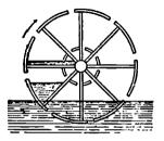
Instead of the wedges of Vitruvius' tympanum, Lafaye's tympanum has cylindrical partitions following the developables of a circle. The angles are economized. The water, entering into the wheel, no longer is lodged in the angles. Thus the shocks are reduced, and so, by the same token, is the loss of labor. Here, I am reproducing the perhaps Hegelian figure of Lafaye's tympanum (1717).
