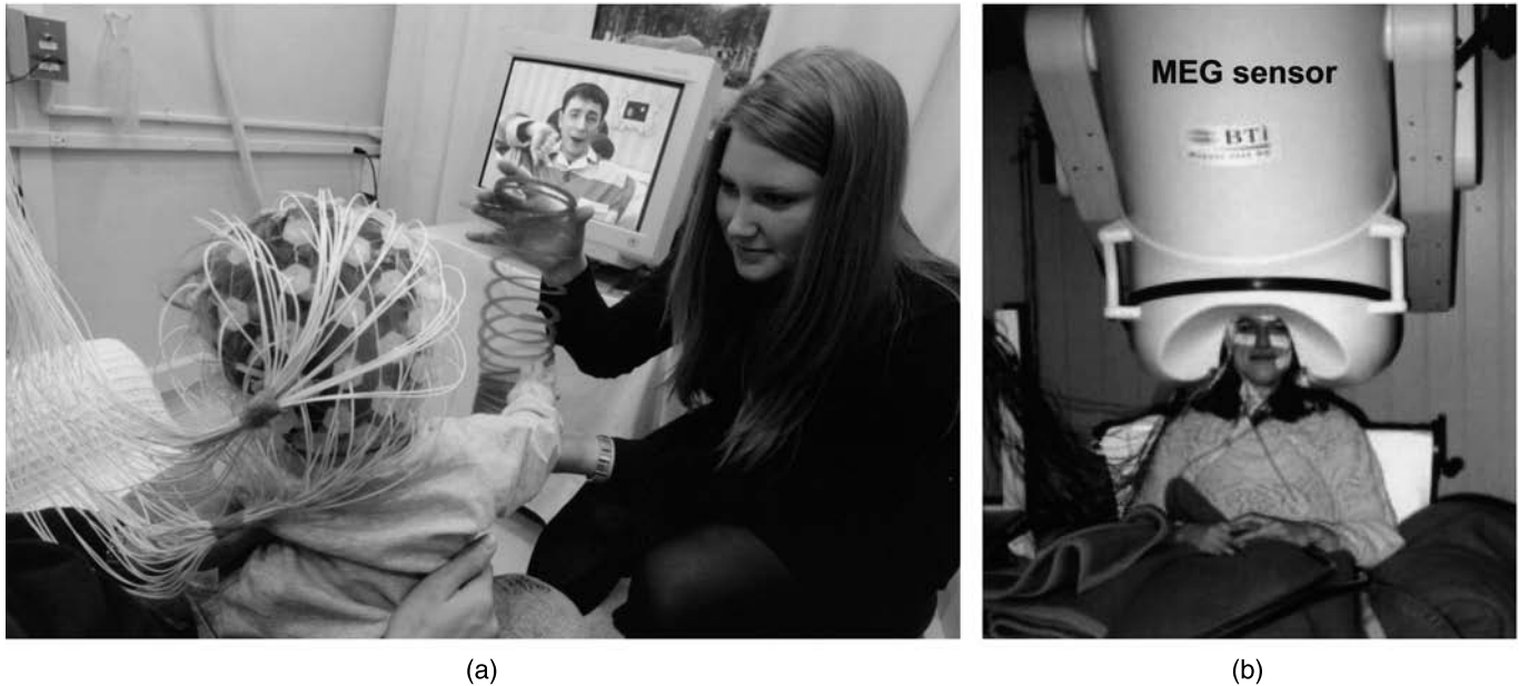
Figure 7.3 (a) An EEG/ERP testing session showing a 9-month-old child seated on her mother's lap and being entertained by an experimenter during a passive auditory oddball paradigm. ERPs are recorded from 62 scalp sites (64 in adults) using the Geodesic Sensor Net (Electrical Geodesics, Inc., Eugene, Oregon). (b) An adult subject in a MEG laboratory. Pictured is a whole-head neuromagnetometer (MAGNES 2500, 4D Neuroimaging, San Diego, CA) inside a magnetically shielded chamber. The device houses 148 detection coils (magnetometers), forming a helmet-like array. It is sensitive to changes in magnetocortical activity, having temporal resolution in the range of milliseconds.
