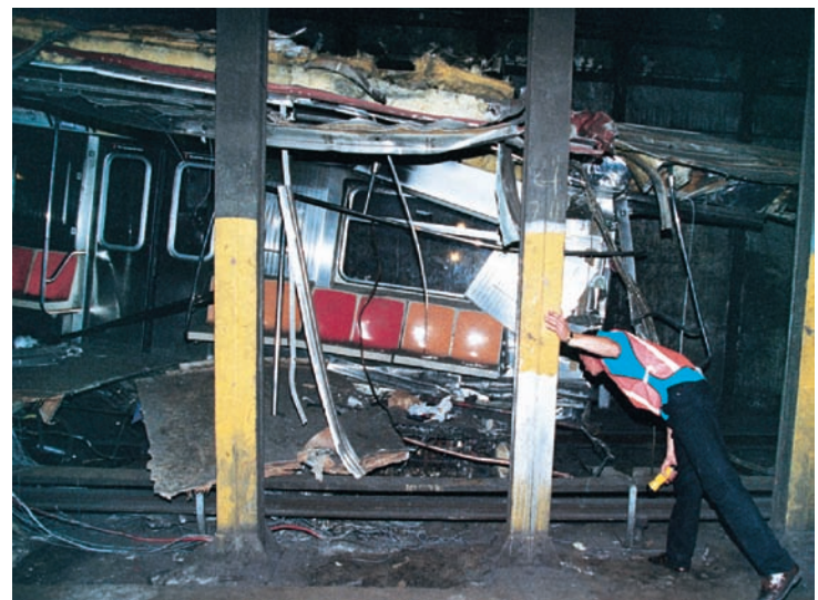
Alcohol is often implicated in vehicular accidents. The driver of this New York subway train, which derailed, killing 5 and injuring over 100 people, was intoxicated. (Corbis Images.)
