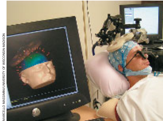
Transcranial magnetic stimulation activates and deactivates regions of the brain with a magnetic pulse, temporarily mimicking brain damage.
