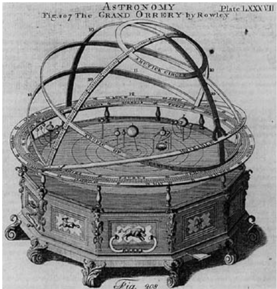
Grand orrery by John Rowley. Orreries, mechanical instruments prized by wealthy amateur astronomers and public lecturers, reproduced the motions of the heavenly bodies according to the Copernican heliocentric theory. (Courtesy Bettmann Archive)
