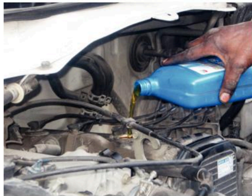
▲ Figure 12.4.1 Oil reduces friction between moving parts
