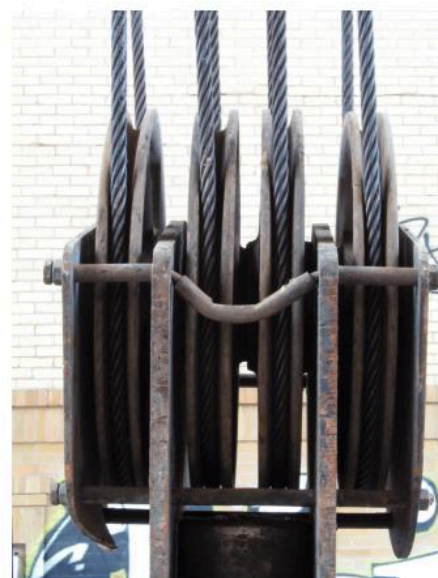
▲ Figure 12.2.6 Multiple pulleys are often put together as pulley blocks
