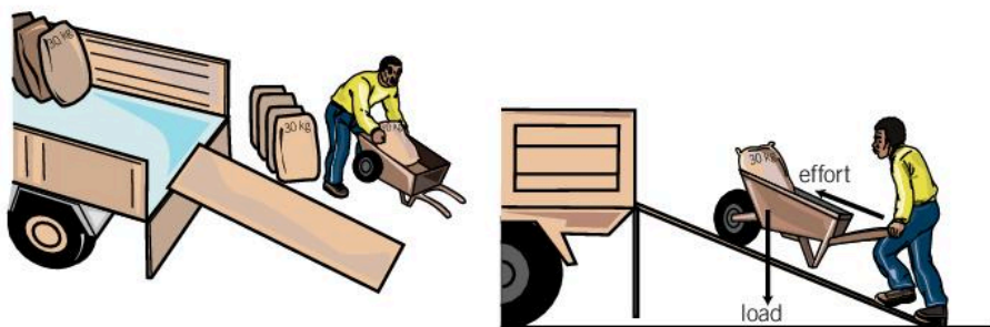
▲ Figure 12.2.1 A ramp is an inclined plane and makes it easier to load things into lorries
