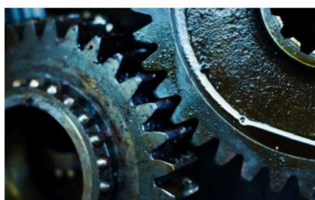
▲ Figure 13.6.2 Oil and grease prevent steel from coming into contact with moisture and air
