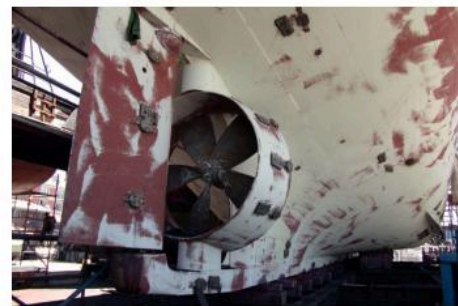
▲ Figure 13.6.7 Zinc is sacrificed to prevent the iron from rusting
