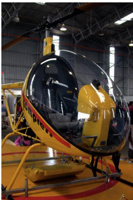
▲ Figure 13.2.3 This helicopter windscreen is made from perspex
