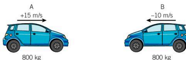
▲ Figure 10.4.4 The momentum of the cars is different in both size and direction
