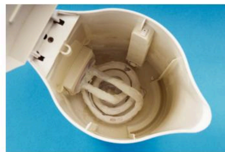
▲ Figure 14.7.1 Lime scale is deposited on heating elements
