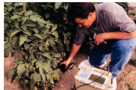
▲ Figure 16.2.1 Testing the water content of soil using an electronic soil moisture probe
