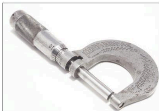
Micrometer screw gauge: measures thickness to the nearest 0.01 mm
