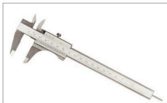
Vernier caliper: measures internal and external distances to the nearest 0.1 mm
