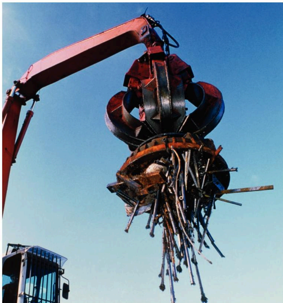
A large magnet is used to separate magnetic metals from other waste at the recycling plant
