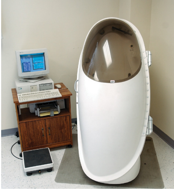
FIGURE 3.3 A Bod Pod, which carries out ADP.
