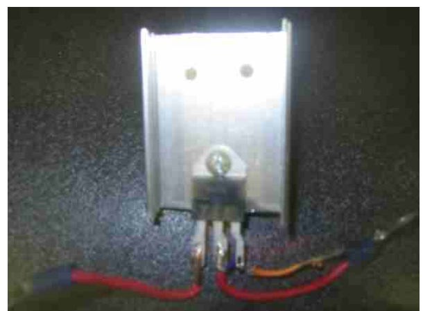
SCR's High amp w/heat sink aluminum
