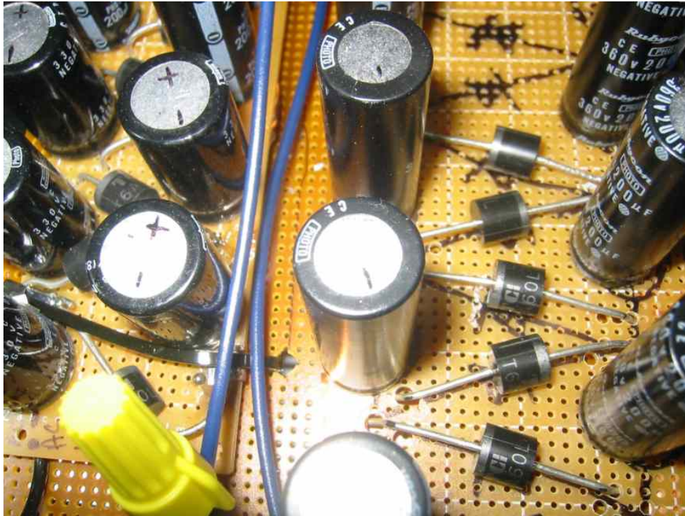
Capacitor's rated at 360 V x 200 uf, Diodes rated at 400 v x 6 amps
