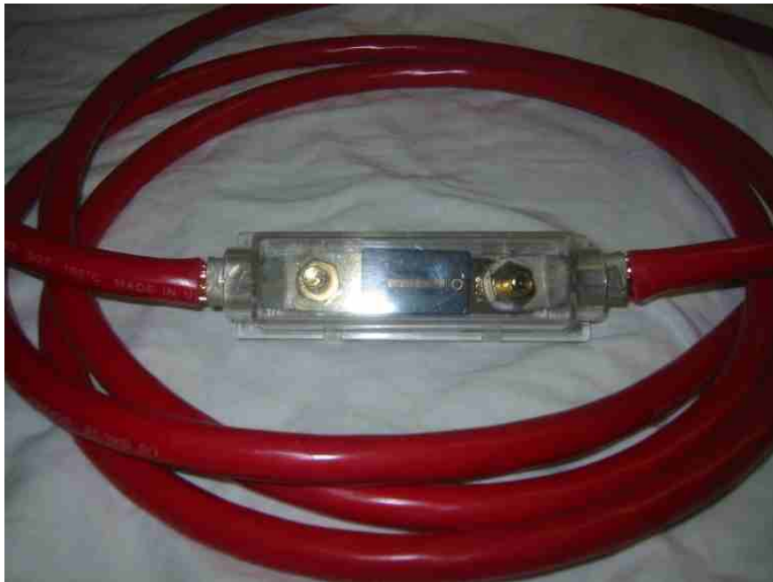
Fuse Box for 12 vdc line
