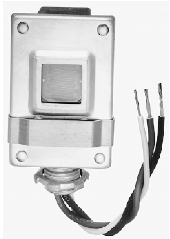
Fig. 2 Exterior photocontrol This unit, shown approximately actual size, is inexpensive and rugged. The sliding metal strip on the cover acts as a mask to reduce the sensitivity of the cell behind the window. The on-off light level ratio is fixed.
