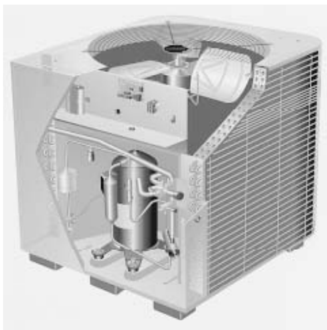
Fig. 1 Air-cooled condensing unit for a residential-sized split system This is typical of units of all sizes. It contains the compressor and its accessories, a large condenser coil, and one or more fans to draw air through the coil. Refrigerant lines connect it to one or more evaporator units inside the building.
