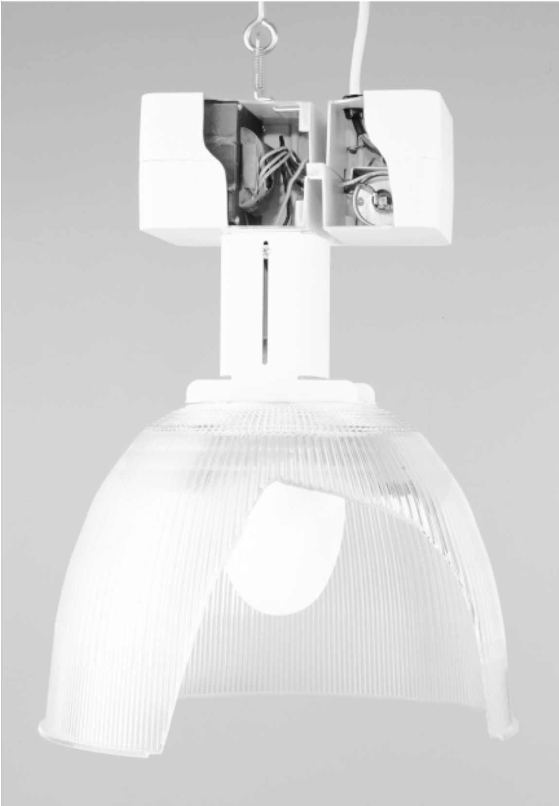
Fig. 1 Typical HID light fixture The ballast is in the upper left compartment. The capacitor and ignitor (if any) are in the other compartment. The two compartments are separated by an air space to isolate the heat of the ballast. The slot and set screw allow the height of the lamp socket to be changed, as a means of adjusting the light distribution pattern. The reflector should be made of glass if any light is intended to pass through it. Plastic diffusers are darkened by the ultraviolet light and heat of HID lamps.
