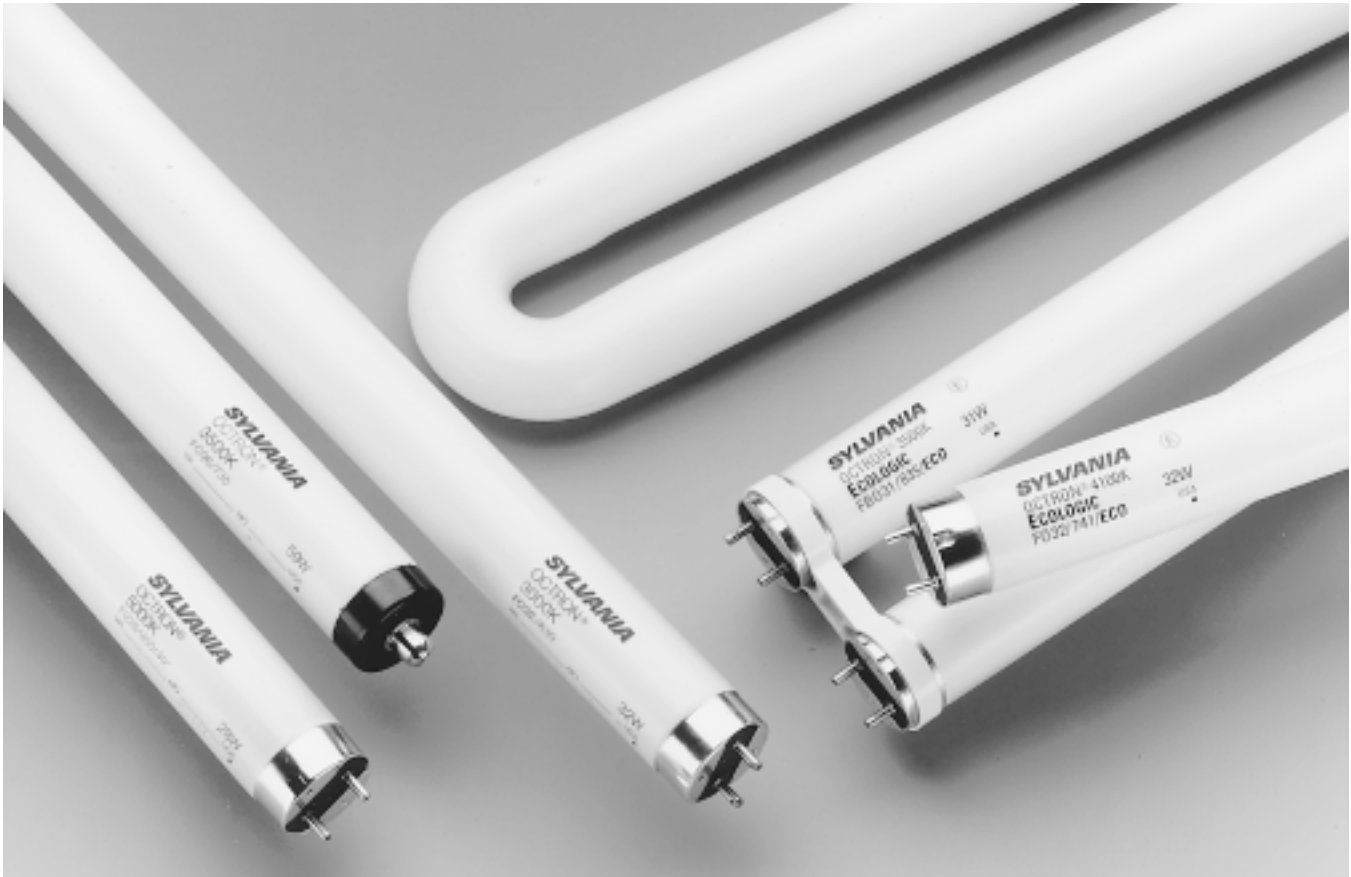
Fig. 1 T8 lamps These lamps have high efficiency and very good color rendering. They fit in the same fixture dimensions as the most common older lamps, but they are not interchangeable with the older lamps. Consider these along with high-efficiency ballasts.
