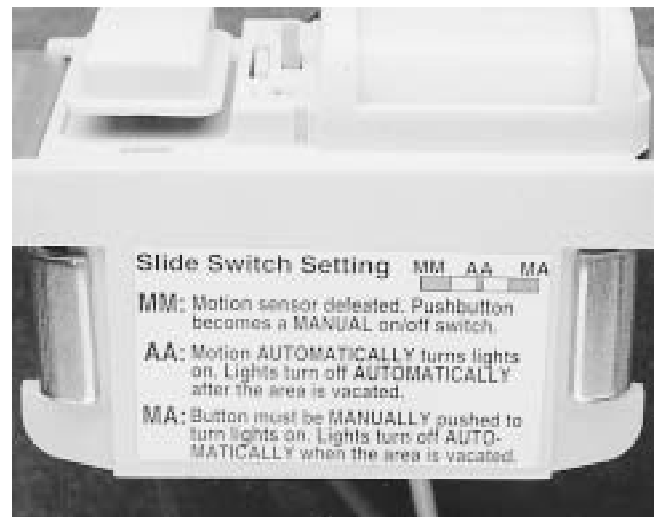
Fig. 7 Override options This sticker explains the override modes that are selected by the switch in Figure 6. Option AA is the one to use in most applications. Option MA is efficient, but has few applications. Option MM abolishes the benefit of the sensor. The sticker becomes inaccessible, and hence useless, when the switch is installed.
