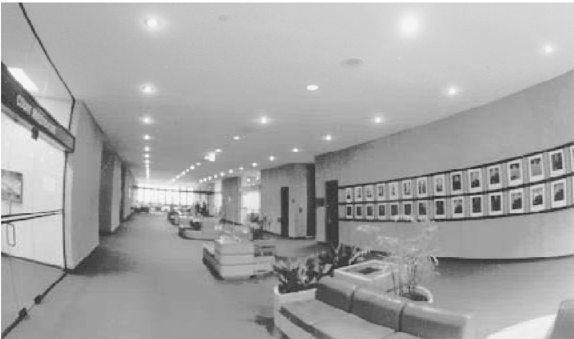
Fig. 2 Downlight abuse in a courthouse Downlights are used as the only source of illumination in this large courthouse lobby. Most of the light is absorbed in the carpet, making this large space gloomy. Note the dark walls, including the portraits of the learned judges. Compare the brightness of the wall in the office at left, which is illuminated with conventional fluorescent ceiling fixtures.
