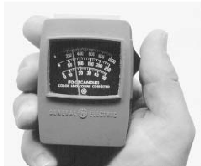
Fig. 1 Footcandle meter The meter is used to measure “illuminance.” It is the only measuring instrument that you need for most applied lighting efficiency work. Being an older model, this meter indicates in units of footcandles. Newer models indicate in units of lux.
