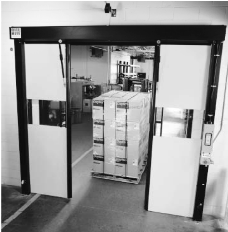
Fig. 2 Horizontally rolling quick-acting door This type quickly provides clearance for tall, narrow loads. The bottom edges of the doors are not restrained, so the struts seen in front of the door are installed to hold the center edges in alignment.
