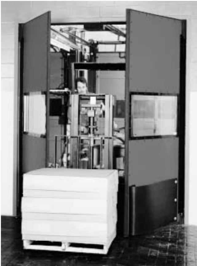
Fig. 1 Impact door As the name implies, this type of door is designed to open by being pushed. The door survives by being light and strong. Plastic bumpers at the bottom of the door absorb much of the shock. The safety issues are obvious here.
