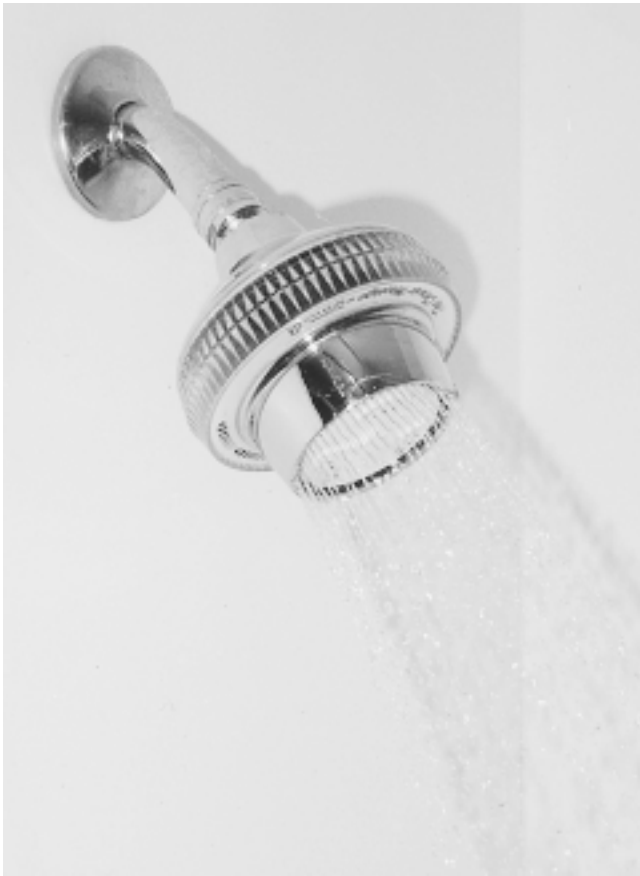
Fig. 3 Versatile and amusing, but not highly efficient This shower head provides a variety of spray patterns, including a pulsating spray. Some of the patterns have higher flow rates. The pattern is selected by rotating the large outer ring, which is somewhat awkward.
