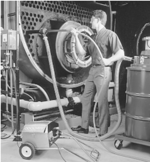
Fig. 1 Cleaning the firesides of a firetube boiler This job is dirty, but not too difficult. The vacuum cleaner attachment, at right, is the largest part of the equipment.
