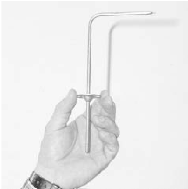
Fig. 1 Pitot tube This pitot tube is easily installed through a small hole in a duct. Additional hardware is needed to convert the pressure to a control signal. The pressure generated in the tube is very small at low air flow rates, limiting accuracy.
