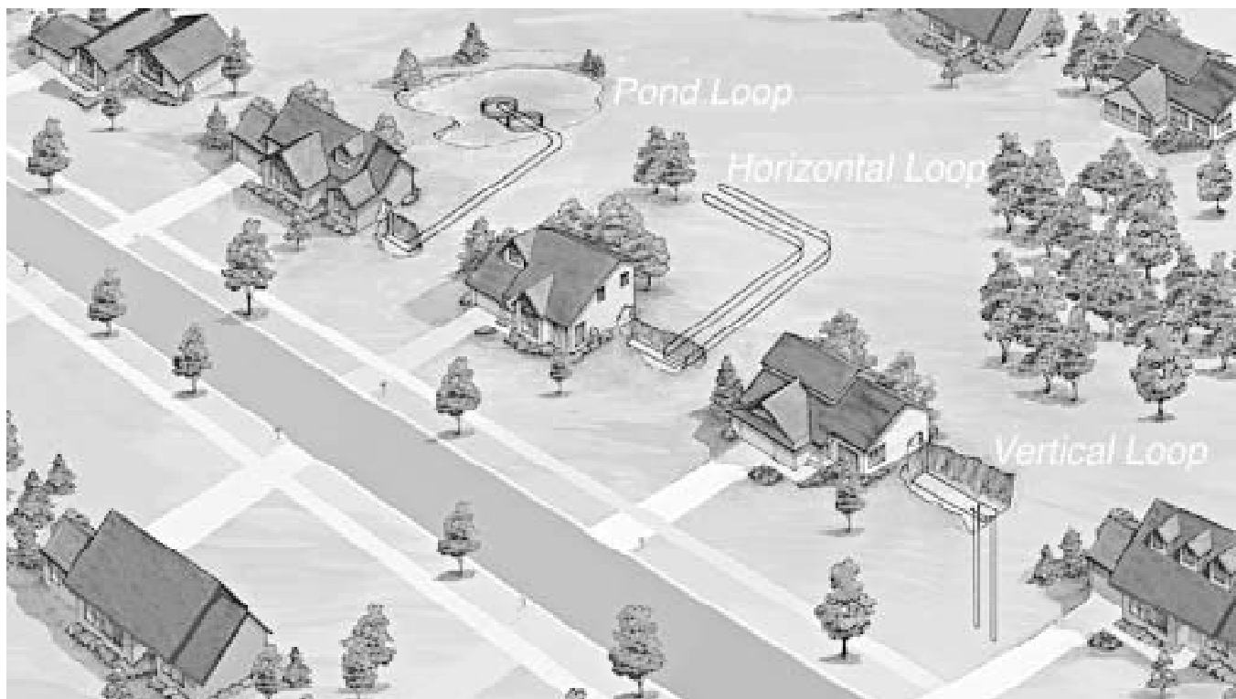
Fig. 1 Alternative heat sources and heat sinks These improve the efficiency of cooling by lowering the average condensing temperature, especially during periods of high cooling load. They improve the average heating efficiency of heat pumps, especially in colder climates.
