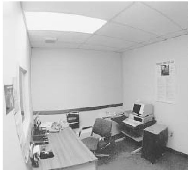
Fig. 1 A work station with serious veiling reflections A person working at this desk is subject to severe veiling reflections from the large light fixture, and from the illuminated area of wall under the light fixture. When the person turns around to work at the computer, he sees strong reflections from the surface of the monitor.
