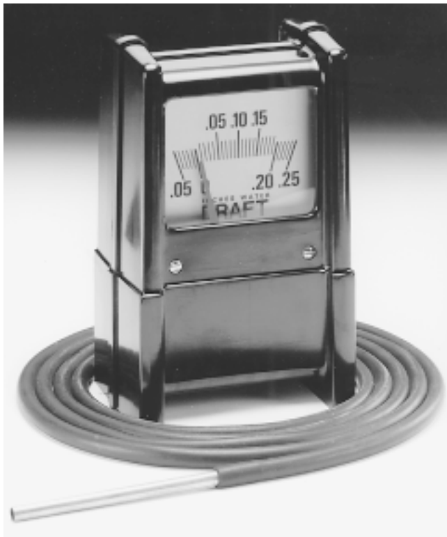
Fig. 3 A portable draft gauge This inexpensive but sensitive unit can be used to measure draft at any point in the boiler system.
