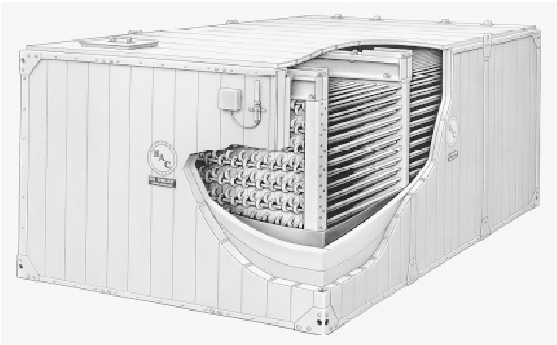
Fig. 8 External-melt ice storage unit This is a tank full of water that is filled with freezing coils. The coils may be cooled by glycol from a chiller, or they may be cooled by direct expansion. Avoiding ice bridging between the coils and maintaining uniform water circulation are important challenges with this type of unit.
