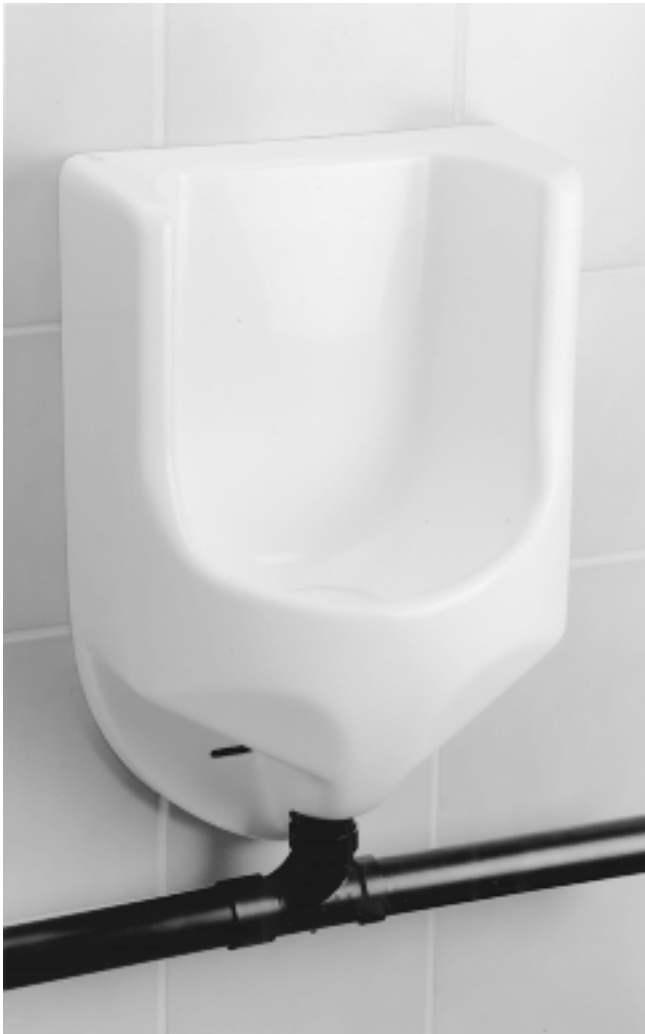
Fig. 2 Waterless urinal This type uses no water for flushing. In the bottom, it has an oil trap that keeps the odor of the urine in the drain trap from entering the space.
