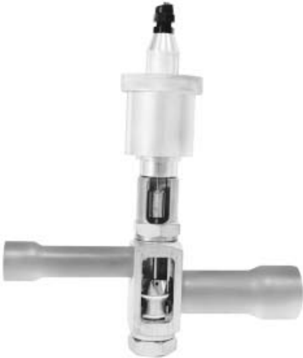
Fig. 20 An “electronic” expansion valve This expansion valve minimizes superheat under all load conditions by changing its throttling behavior. The valve receives input signals from a microcomputer that senses system conditions.
