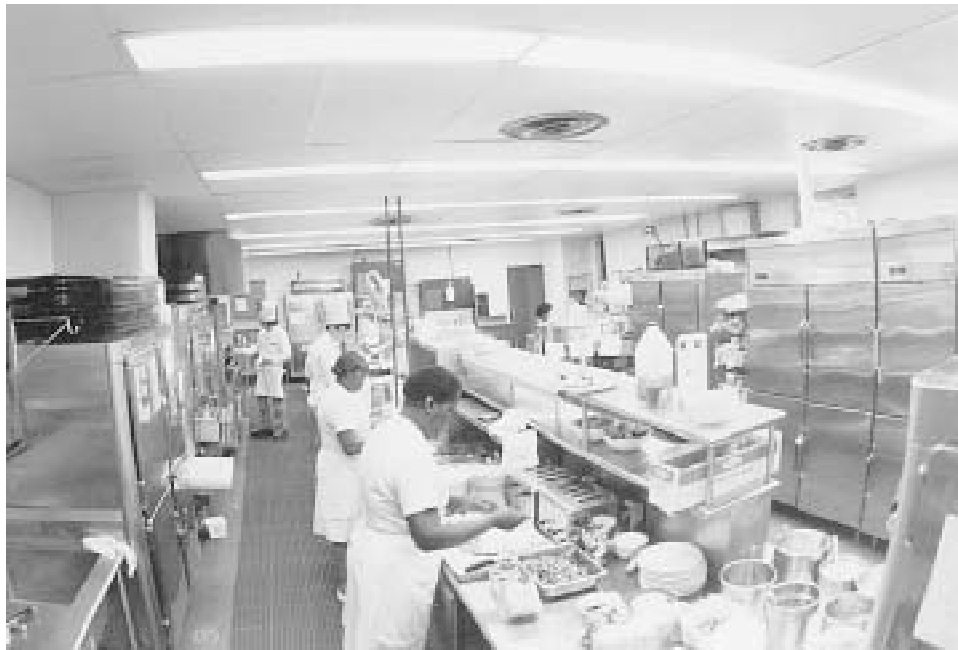
Fig. 2 Some lessons about glare and veiling reflections This hotel kitchen requires a high illumination level throughout the space for food preparation and sanitation. At first glance, the metal surfaces everywhere appear to cause serious glare and veiling reflections. However, the shelves at the rear of the counters shield the work area from most veiling reflections. The work involves a large amount of movement and shifting gaze, which limits the duration of exposure to veiling reflections. The uniformity of the lighting reduces glare by not requiring the cooks' eyes to adapt to different brightness levels as they work. This lighting environment is at the opposite end of the spectrum from those where task lighting is appropriate. With task lighting, each work area must be arranged individually to avoid glare and veiling reflections.
