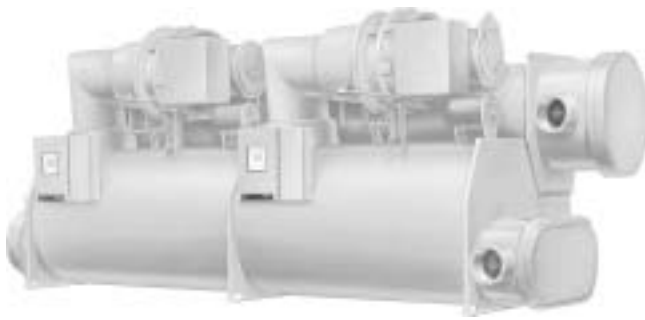
Fig. 9 A large water chiller with two centrifugal compressors This is one way of maintaining efficiency at reduced cooling loads.
