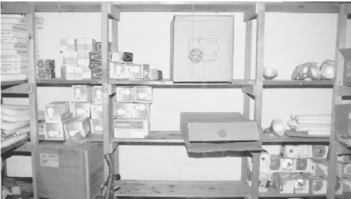
Fig. 1 Lamp stockroom This is what the maintenance staff faces. If there are several types of lamps that will fit into the same socket, the wrong lamps will eventually be installed unless you mark all fixtures with the types of lamps they use.
