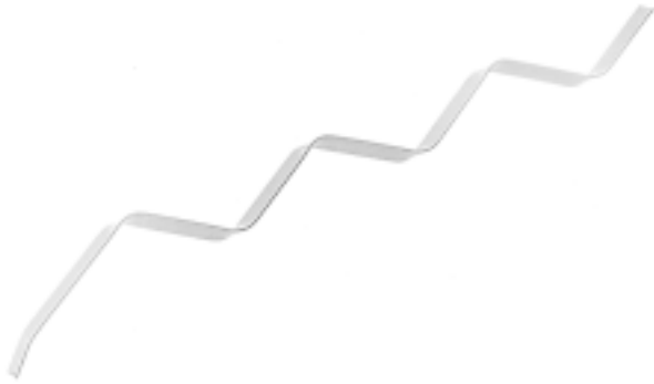
Fig. 1 Typical turbulator This is simply a strip of steel, bent into a shape that holds it within the boiler tube by friction.
