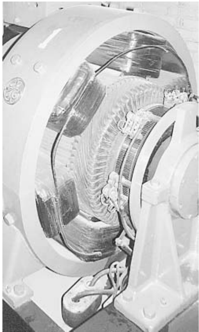
Fig. 17 Direct-current motor This elevator motor clearly shows the major components of a DC motor. The six stator poles and the rotor windings are energized by electric current. Current reaches the rotor windings through carbon brushes that slide over the commutator on the near end of the rotor. The commutator keeps the magnetic field of the rotor stationary in space as the rotor turns. Note that there is a rotor brush corresponding to each stator pole. The rotor and stator fields remain aligned for maximum torque. Speed and torque are varied by changing the current in the windings.
