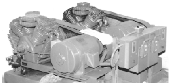
Fig. 6 High-torque application This reciprocating air compressor requires full torque almost immediately after it starts. This is because the force needed to compress the air in the cylinders is almost independent of the speed.
