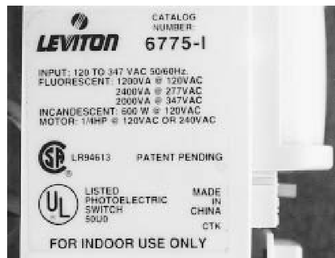
Fig. 8 Critical electrical information This infrared switch can control different kinds of electrical equipment, including motors, but the capacity ratings are different for each kind.
