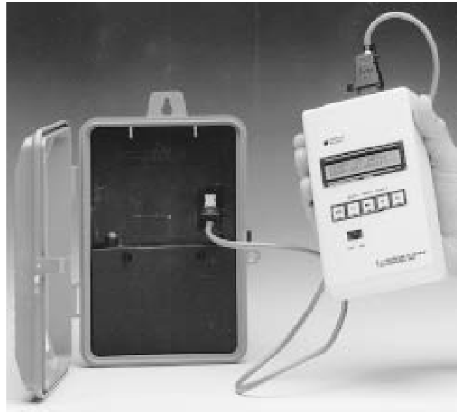
Fig. 6 Remote-setting time control This is a handy feature for some applications. However, an override is needed at the point where this control affects people.
