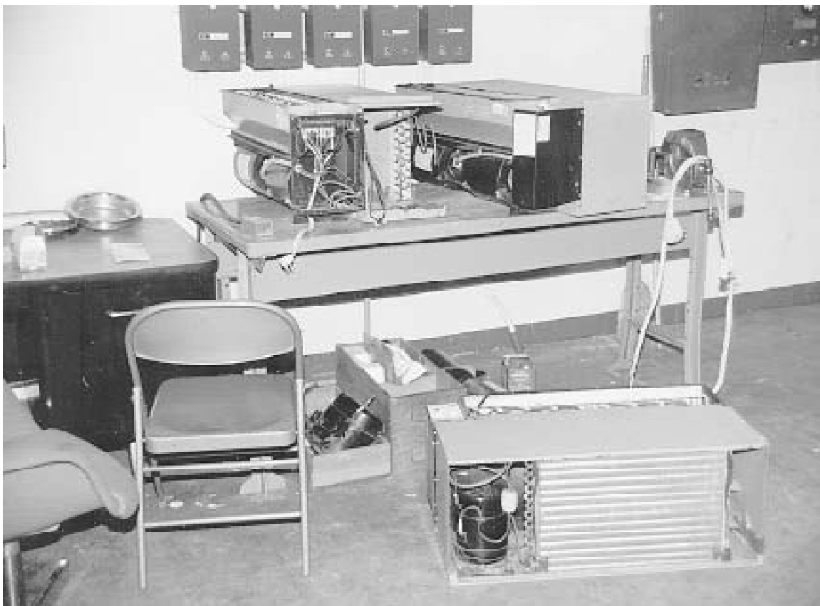
Fig. 1 Where air conditioners go to die The air conditioners in this large hotel typically fail within a year or two after a compressor is replaced. We can see why. There is no equipment here for properly purging the units after the repair is made.
