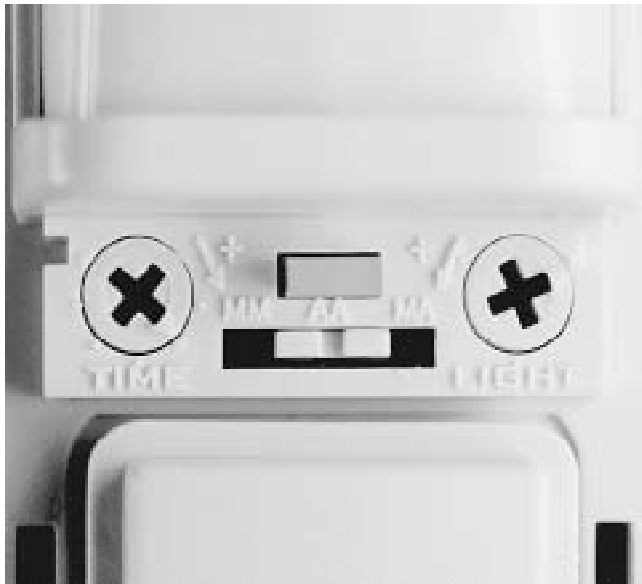
Fig. 6 A good set of features in an infrared sensor The screw on the right adjusts the daylight level that keeps lights turned off. The screw on the left adjusts the turn-off delay. Both require trial-and-error to set. The slide switch in the middle selects the override mode, explained in Figure 7. The switch plate must be removed to change any of these settings, which is an important safeguard. The little rectangular light amuses occupants by blinking when the sensor detects motion.
