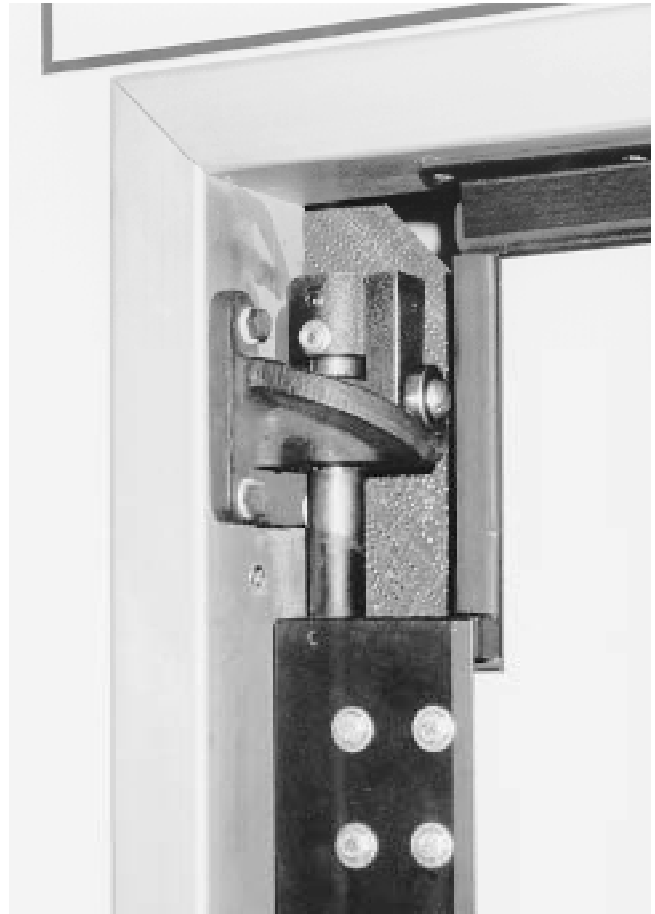
Fig. 2 Centering hinge This is the most common type of centering device for impact doors. The weight of the door is carried by a roller fitting, which falls by gravity into a V-notch. This aligns the doors accurately enough to engage the infiltration seals. The hardware has virtually unlimited life. The infiltration seal on top of the door must accommodate the rising of the door as it opens.
