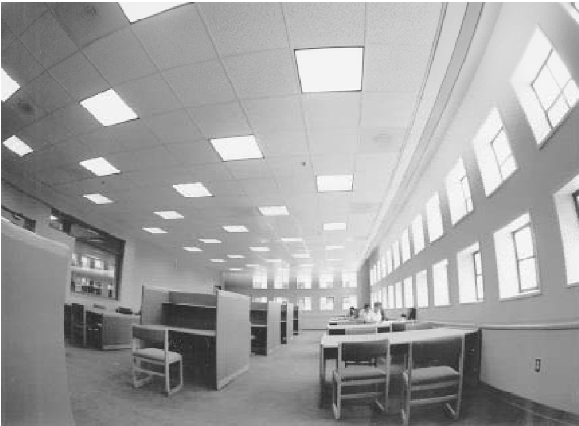
Fig. 2 Task lighting challenge No. 1 This is a large reading room in a public library. The present light fixtures shine mostly on the carpet and on empty tables. Daylighting is not being exploited. All reading occurs at individual furniture units, which can be moved and reoriented. There are many windows, and they extend high on the wall. What would you do to make this lighting efficient and pleasing?
