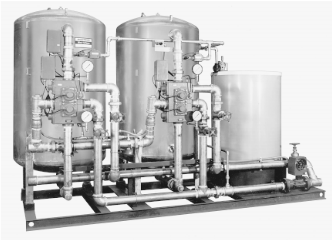
Fig. 3 Water softening system This is used to treat makeup water before it enters the boiler system. It replaces minerals that cause scaling with other materials that remain dissolved in the boiler water.
