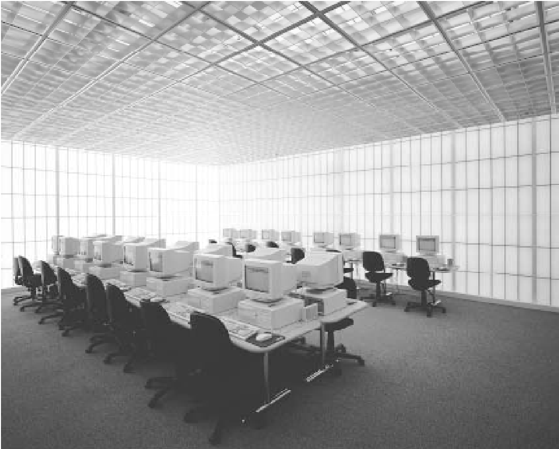
Fig. 6 A challenging translucent wall application In this computer classroom, the students are required to face the translucent walls for long periods. Avoiding glare must be a major design issue here. The potential for glare, as well as the potential for saving energy by daylighting, is determined by the transparency of the wall. The dominant factor in selecting panel transparency is whether the exterior of the panels is exposed to direct sunlight. The relative brightness of the walls and the computer screens must also be considered. The ceiling is full of light fixtures. If the walls are too bright, the lights will be kept in operation to compensate.
