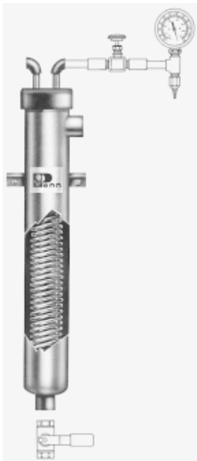
Fig. 5 Sample cooler This is valuable when taking water samples from a boiler that operates above boiling temperature. Without it, tests will show concentrations higher than they actually are. It also reduces the risk of scalding when taking samples.
