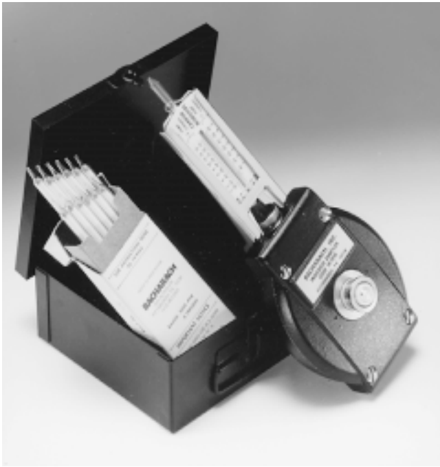
Fig. 5 Chemical carbon monoxide tester The simple device on the right draws a flue gas sample through a glass tube containing a chemical that reacts with carbon monoxide to change color. Each tube is used one time. By using different chemicals, the device can test for other flue gases.
