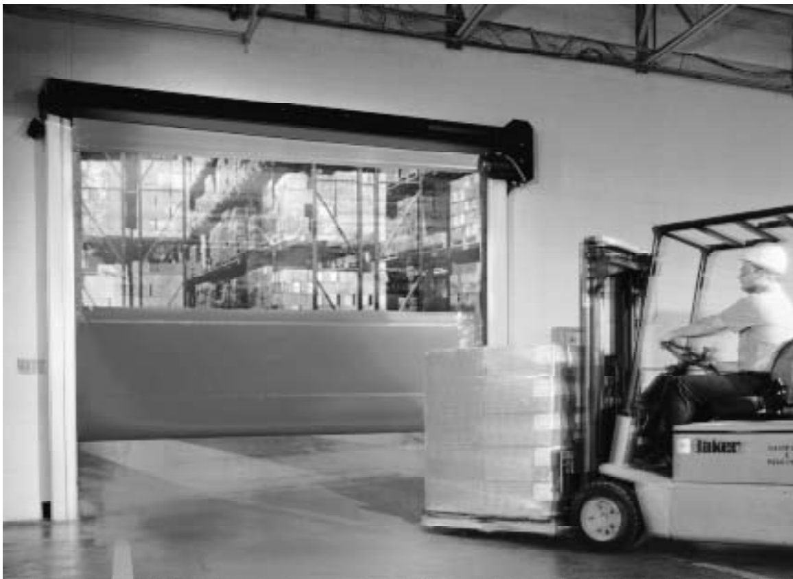
Fig. 1 Vertically rolling quick-acting door The motor that rolls up the door is on the upper right side of the frame. A large window is needed for safety. The driver has a view of the complete width of the floor on the other side as soon as the door starts to open.
