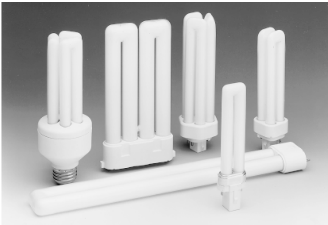
Fig. 2 Compact fluorescent lamps These are available in smaller wattages than common conventional lamps. Their small physical size allows them to concentrate light on small task areas, and they can be mounted in aiming fixtures. For these reasons, they hold the key to using fluorescent lighting in task lighting. However, they are less efficient, per watt, than the larger lamp styles. The emerging multitude of lamp wattages and base types is creating a future standardization problem that will probably cause many of the present types to become obsolete.
