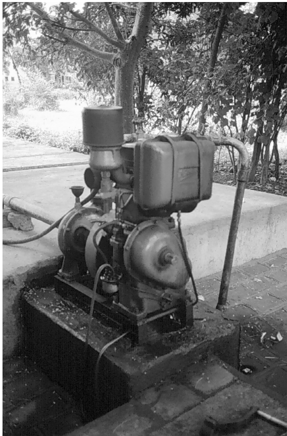
Figure 1: Diesel-driven pump ©Practical Action
