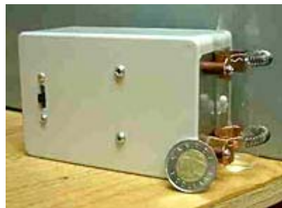
Constant heat, constant agitation of the titration sample (note the test tube at the right end of the box)
