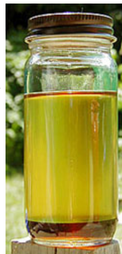
Freshly made biodiesel, 20 minutes after processing
