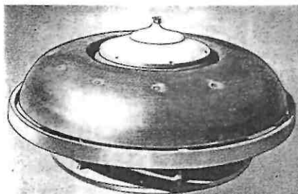
(b) Machine with upper air-intake cone removed to show inner air-distributor cone.
