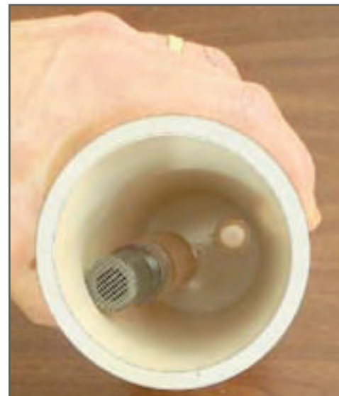
Looking up towards the top cap of the bubbler. Notice gas exit port at about two o'clock.
