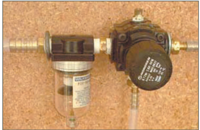
Water filter (left) and regulator (right)
