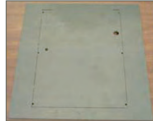
The PVC end plate with holes drilled for the gas inlet and outlet and the pressure screws
