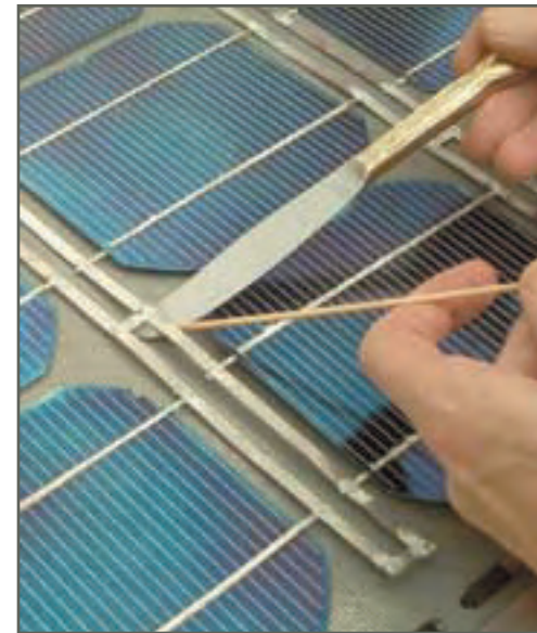
Dab silicone under the bus wire to hold the strings of cells in place
