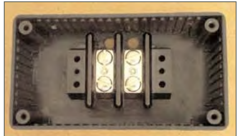
The power take-off box, parts (above) and assembled (below)
