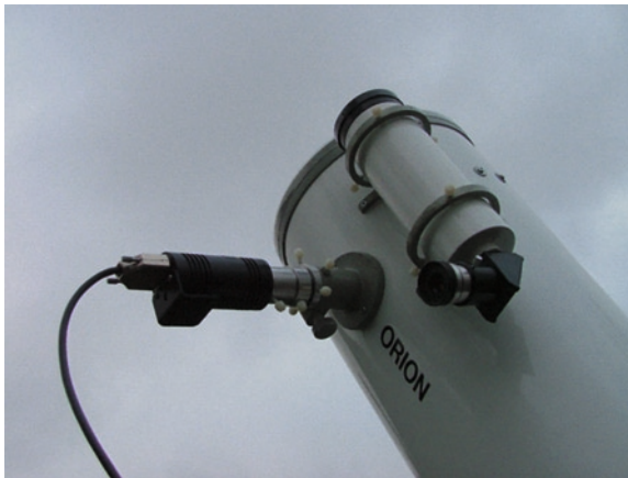
Fig. 10.5. Starlight Xpress CCD camera with stop ring in position (Photo by the author).
