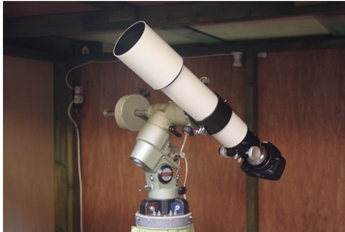
Fig. 9.8. Michael Clarke's 80 mm refractor, Canon camera, and Vixen mount (Credit: Michael Clarke).
