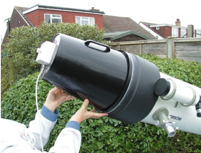
Fig. 10.4. Light bin for obtaining flat fields (Photo by the author).
