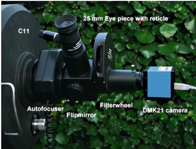
Fig. 9.4. John Sussenbach's Celestron C11 and imaging attachments (Credit: John Sussenbach).
