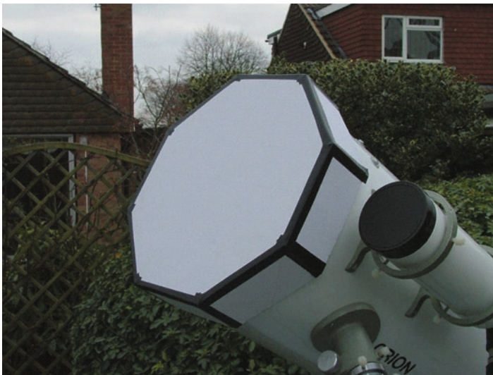
Fig. 10.3. Light-tight cap for obtaining dark frames (Photo by the author).
