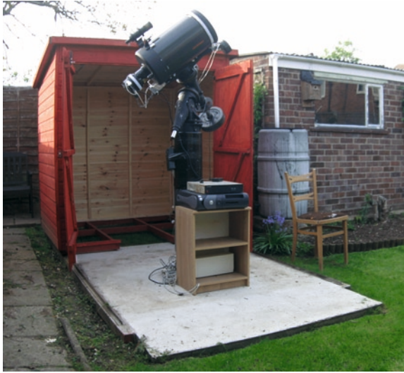
Fig. 7.5. Nick James's roll-off shed observatory ready for use with pillar extended (Credit: Nick James).
