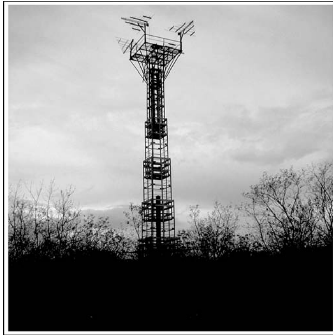
Figure 20.3: A picture of the antennas of the RFI monitoring system of GMRT. Four log-periodic antennas are mounted on a tower of 20 m height in the E-plane directed along East, West, North, and South directions.
