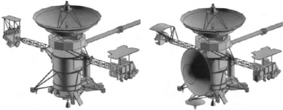
Outlines of the Comet Rendezvous and Asteroid Fly-by (left) and Cassini–Huygens (right) spacecraft as envisaged using the generic Mariner Mark 2 configuration
