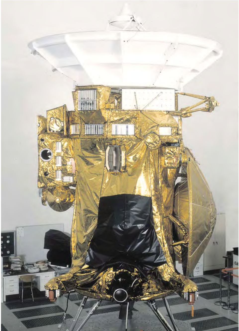
Ready: the Cassini spacecraft with the Huygens probe attached.
