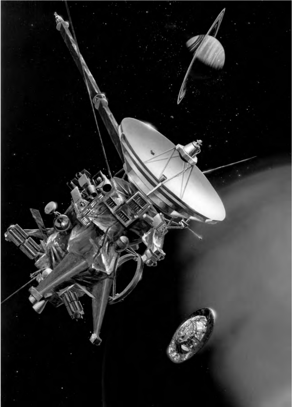
An artist's impression of Cassini releasing the Huygens probe. Note that a certain licence has been taken concerning the range from Titan when this occurs.
