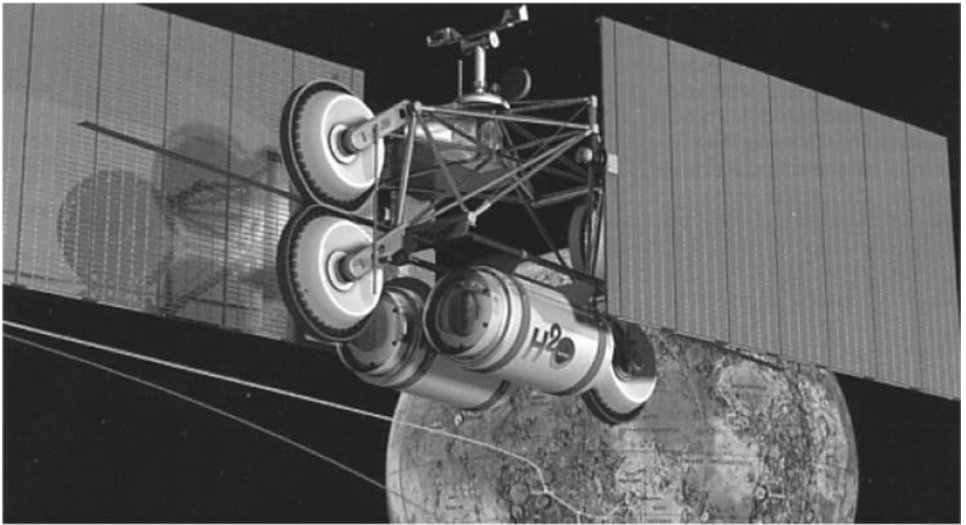
FIGURE 4.10. A lunar space elevator reaching the L_1 Lagrangian point of the Earth–Moon system. (Courtesy Moon Base Conference.)
