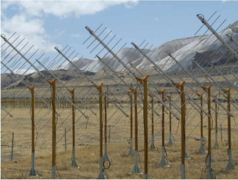
Figure 7.6 The 21 Centimeter Array (21CMA) in the Xinjiang province of western China, consisting of approximately 10 000 dipole antennas.
