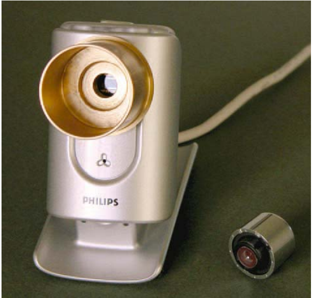
Figure 3.1. Philips Toucam Pro II with 1.25-inch adapter replacing the lens. Note on the rear of the original lens is an infrared block filter.
