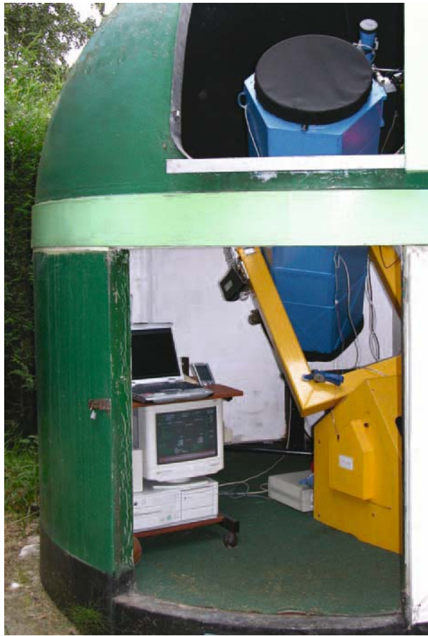
Figure 9.3. 16-inch telescope inside the observatory. A classical dome is ideal for blocking local light pollution. The lower computer controls the telescope while the upper laptop operates the CCD camera.
