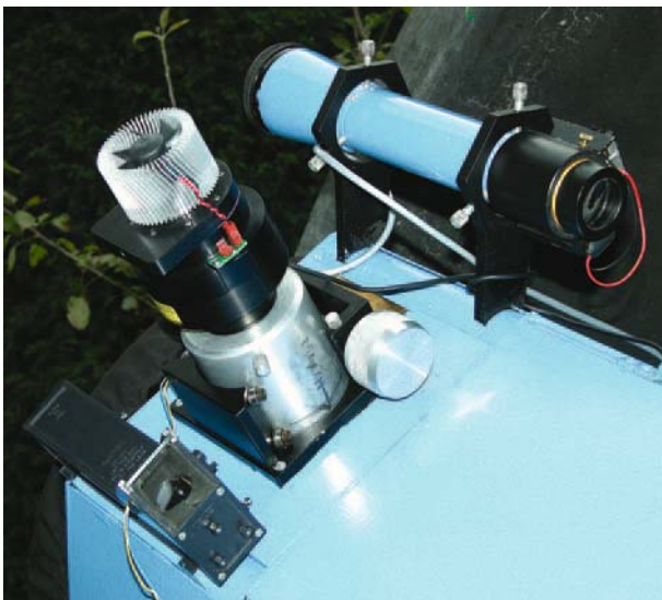
Figure 9.4. FLI Maxcam CCD camera. Note the large Crayford focuser. Pencil marks on the side of the focuser might look crude but they indicate the approximate focus position.
