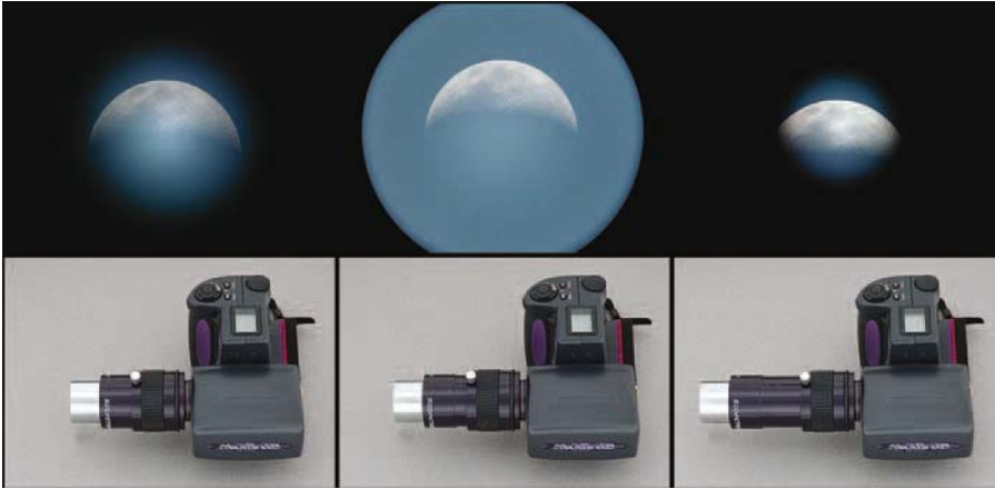
Figure 2.10. Adjusting the Nikon 990 camera field stop distance at minimum zoom to match the ScopeTronix 40mm eyepiece eye relief. From left to right: camera too close to the eyepiece lens, camera at best position and camera too far from the eyepiece lens. Images of the Moon were taken during daylight to show vignetting. With the ScopeTronix 40mm eyepiece you can adjust the distance of the camera from the top lens of the eyepiece.
