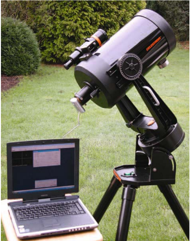
Figure 3.4. Toucam Pro II attached to the visual back of a Celestron C8 – the base of the webcam has been unclipped. Due to a shorter USB cable the laptop PC has to be close to the telescope. If you need to be further away, use a USB extender.
