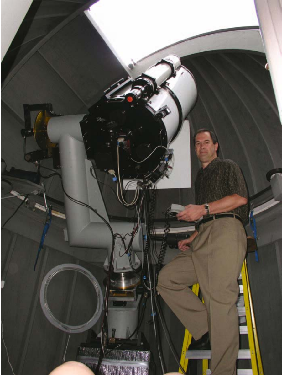
Figure 8.4. Brian Lula with his 20-inch Ritchey-Chretien (RC) telescope and home-built heavy-duty equatorial fork mount. This telescope replaced a personally built 20-inch F/5 Newtonian astrogaph used to take some of the deep-sky images in this chapter. Note the silver wrap on the telescope pier. The pier produced considerable thermals during the night, seriously affecting local seeing. An inch-thick layer of rigid Styrofoam glued all around the pier and further wrapped by aluminized polyethylene bubble wrap improved seeing conditions considerably.
