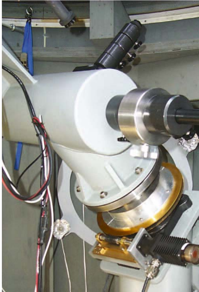
Figure 8.8. A mechanical engineer by profession, it shows in Brian's home-built heavy-duty equatorial fork mount. Home-building a precision-tracking mount is an onerous task. Note the silver wrap insulation on the telescope pier.
