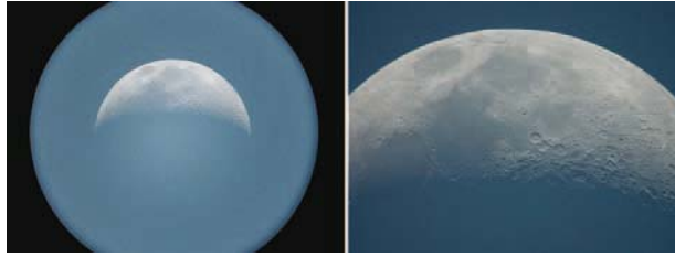
Figure 2.9. Daytime moon images showing vignetting at minimum zoom in the left image and removing it by increasing the camera zoom in the right image.
