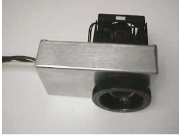
Figure 4.3. Cooled SC modded ToUcam, by Ashley Roecklein.
