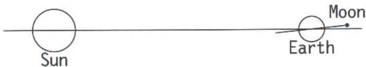
FIGURE A-7. The Moon has an orbit that is tilted slightly against the plane, called the ecliptic, in which the Earth circuits the Sun. In this diagram ( not drawn to scale) we look sideways along the ecliptic, and note that the lunar orbit makes an angle of about five degrees to it, with an orientation that swivels around making alignments of all three bodies possible. An eclipse can only occur if the Moon happens to be crossing the ecliptic when at conjunction (producing a solar eclipse) or opposition (producing a lunar eclipse).
