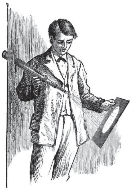
FIGURE 1-13. How to avoid blinding yourself while trying to observe the Sun with a telescope. This nineteenth-century drawing shows how to project an image onto a screen, an invaluable technique for eclipse watchers.
