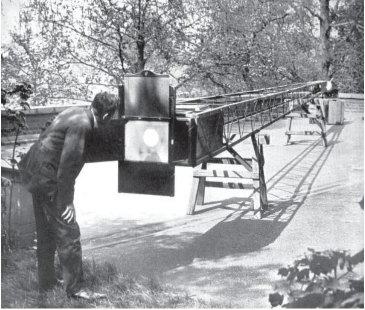
FIGURE 4-4. A heliostat (a rotating mirror used to track the Sun) may be used to reflect an image horizontally into a camera. This is an easier solution than having a long camera tube directed skywards (see Figure 4-5).
