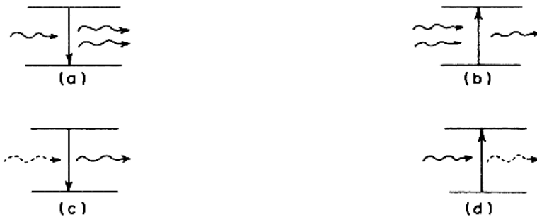
Fig. 7.10. In part (a) a photon of frequency \nu stimulates the emission of a similar photon, while the particle energy drops by an amount \mathcal{E} = h\nu . In (b), the time-reversed process takes place. The particle transits to the higher energy state \mathcal{E} by absorbing a photon. As discussed in the text, spontaneous emission of radiation from a singly excited radiation oscillator (c) corresponds to the time-reversed process of absorption of energy (d) by a particle in its ground state.
