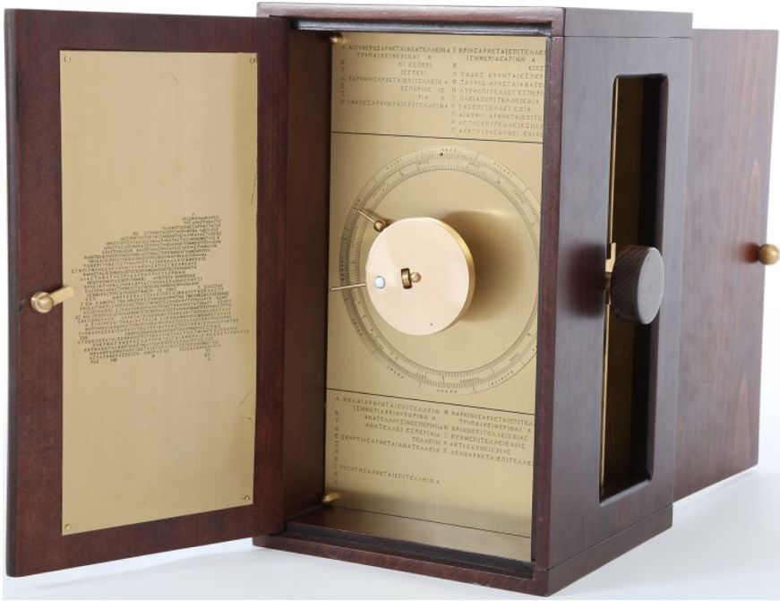
PLATE 3 Modern reconstruction of the front of the Mechanism Pointers carry gold and silver balls representing the Sun and Moon, respectively. The Sun pointer also indicates the day in the Egyptian calendar. The Moon ball rotates to show the changing phase of the Moon. All this is activated by turning the knob at right. Most scholars believe that there were also moving pointers representing the planets but these have not survived. ARISTOTLE UNIVERSITY: ANTIKYTHERA MECHANISM, MODEL V.2. [PHOTO COURTESY OF JOHN H. SEIRADAKIS]
