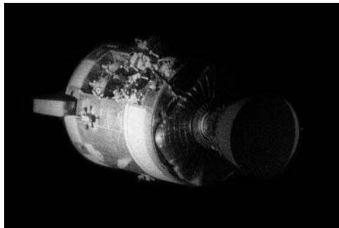
Apollo 13's shattered service module.
