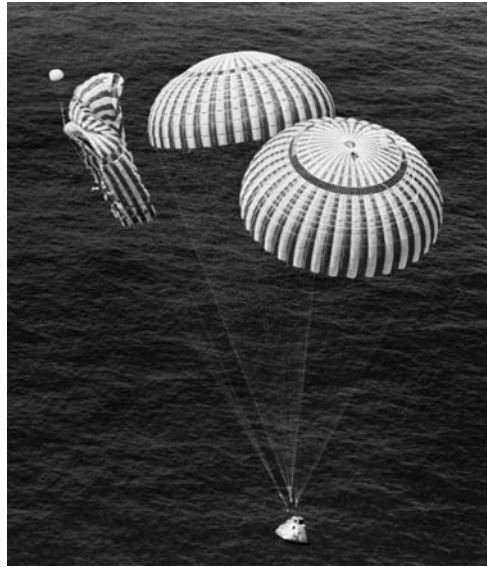
The Apollo 15 CM descends with one of its three main parachutes tangled.
