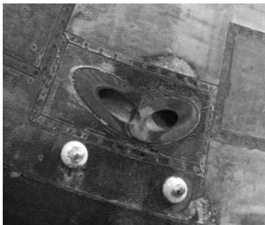
Water and urine dump nozzles below the roll thrusters on Apollo 10’s CM.
