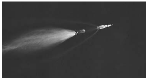
Apollo 11's S-IC stage falls away as the S-II takes over.
