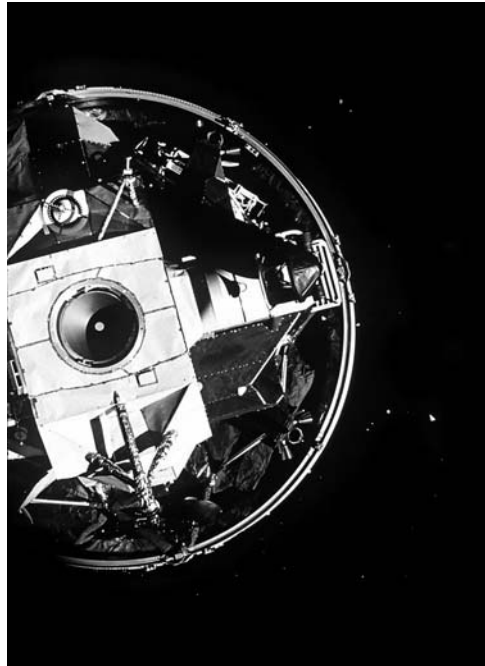
Apollo 15’s lunar module still within the S-IVB and surrounded by a cloud of particles.
