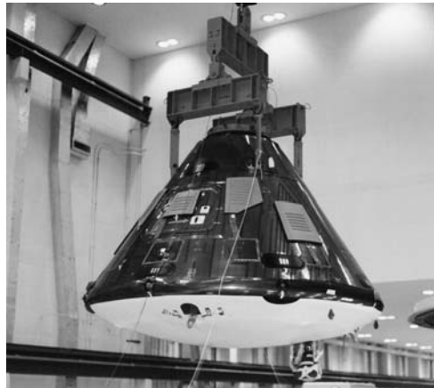
Apollo 17's command module, prior to being mated with its service module.
