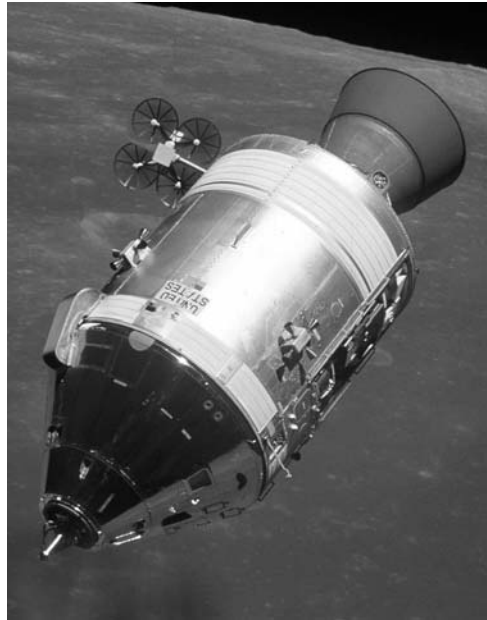
Endeavour , Apollo 15's CSM in lunar orbit. The four dishes of its high gain antenna are visible near the engine bell.
