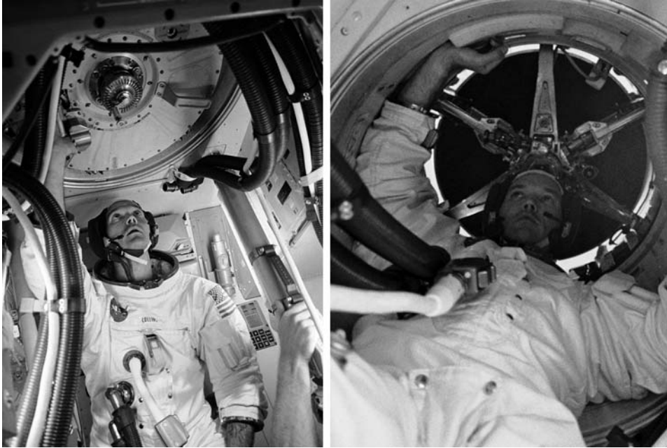
Mike Collins working in the tunnel during training. Left, at the forward hatch. Right, below the probe mechanism.
