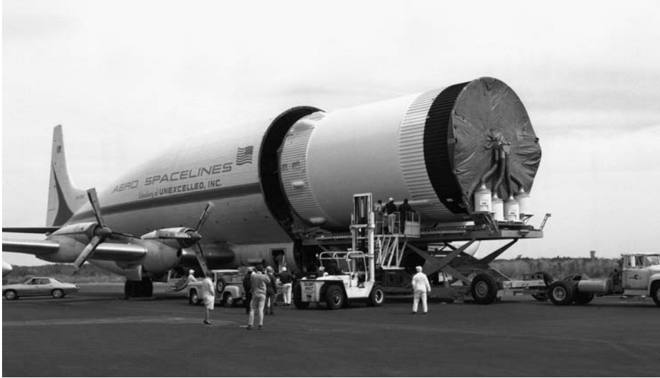
Apollo 12's S-IVB stage during transportation on a Super Guppy aircraft.
